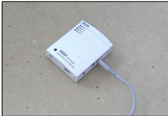
Figura 17. Sensor HOBO H8 RH/Temp/Light/External H08-004-02.
