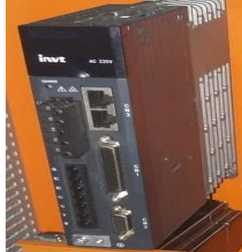
Figura 3. 28: Servodrive INVT SV-DA200-0R1
