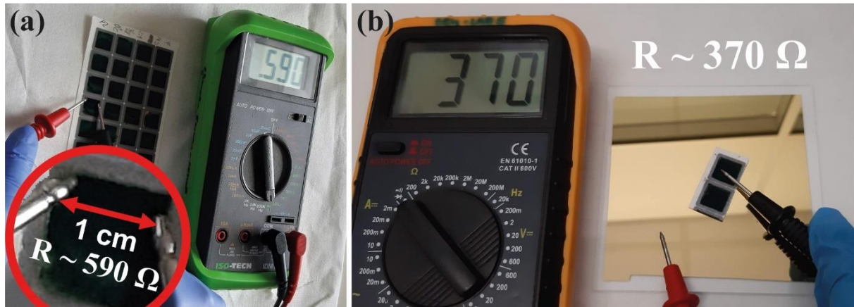
Figure 3.2.1 – (a), (b) Lateral and cross-sectional resistance of the FCP, respectively
