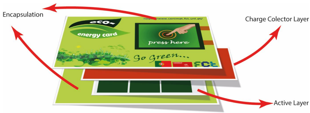
Figure 2.5.1 – Schematic of the devices built, comprehending three layers: the active layer (AL) that has the FCP, the charge collector layer (CCL) which consists of the paper based electrodes and the encapsulation layer, which is also paper-based.
