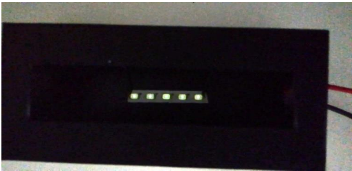
Figure A.5.2 - Instantaneous powering of 5 white LEDs (1.5W).
