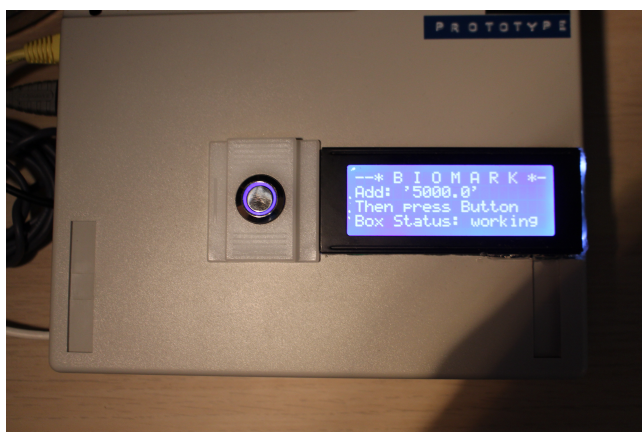
Figure 5.20: Calibration Box waiting the addition of reagent manually.
