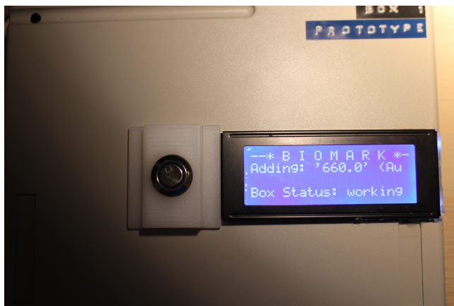
Figure 5.19: Calibration Box adding reagent automatically.
