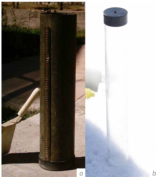
Figure II-1.2.1 Instruments used only in the 1 st HarmoSnow field campaign: (a) TSMS cylinder from Turkey; (b) Plexiglas tube from Italy.
