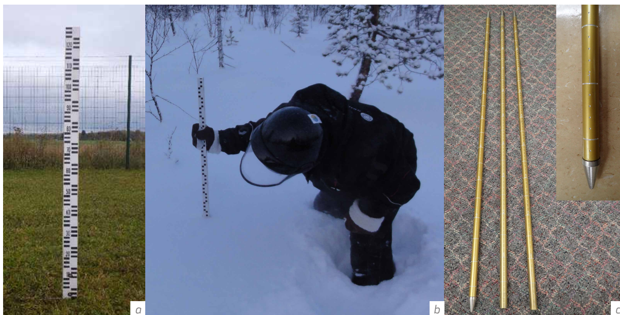
Figure I-1.2.1 (a) Graduated snow stake installed before the onset of a snow cover (Source: ESTEA). (b) Snow depth measurement with a ruler in northern Finland (Source: FMI). (c) An extendible 1-cm-graduated snow rod (Source: ECCC).
