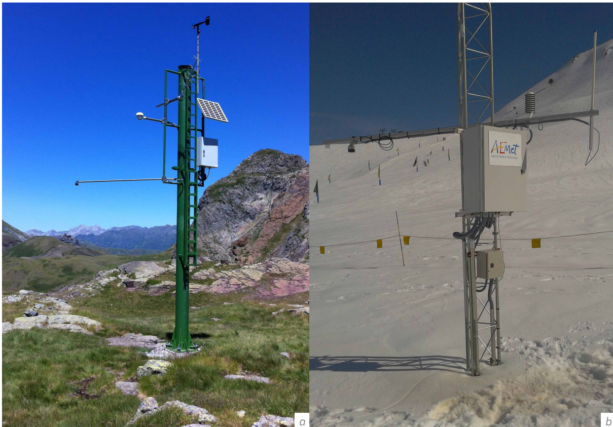
Figure I-2.34.11 Automatic weather stations in the Pyrenees (Spain) operated by AEMET: (a) in Anayet; (b) in Formigal (Source: AEMET and collaborators).
