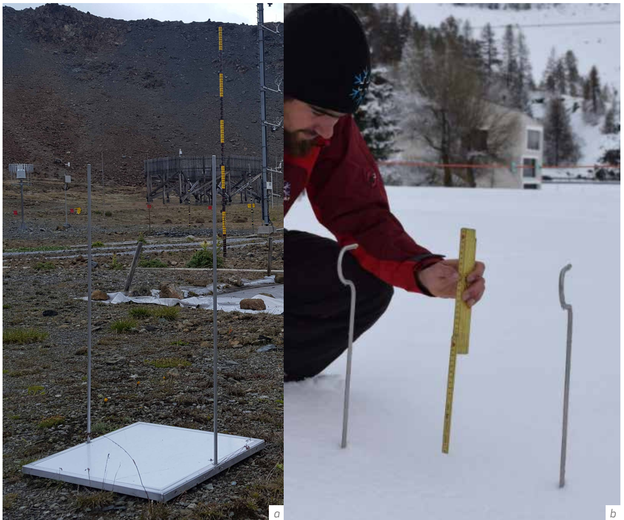
Figure I-2.36.7 (a) Snow board fitted with two 100-cm-long rods so that the board can be located after a snowfall event. In the background a graduated black and yellow snow stake to measure snow depth is visible. (b) An observer measuring depth of snowfall on a snow board (Source: SLF).
