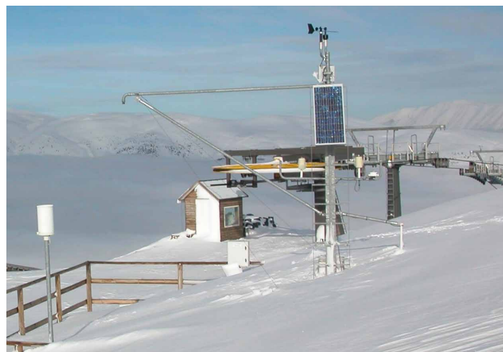
Figure I-2.19.6 Automatic weather station operated by MC, with an ultrasonic snow depth sensor (Source: MC).
