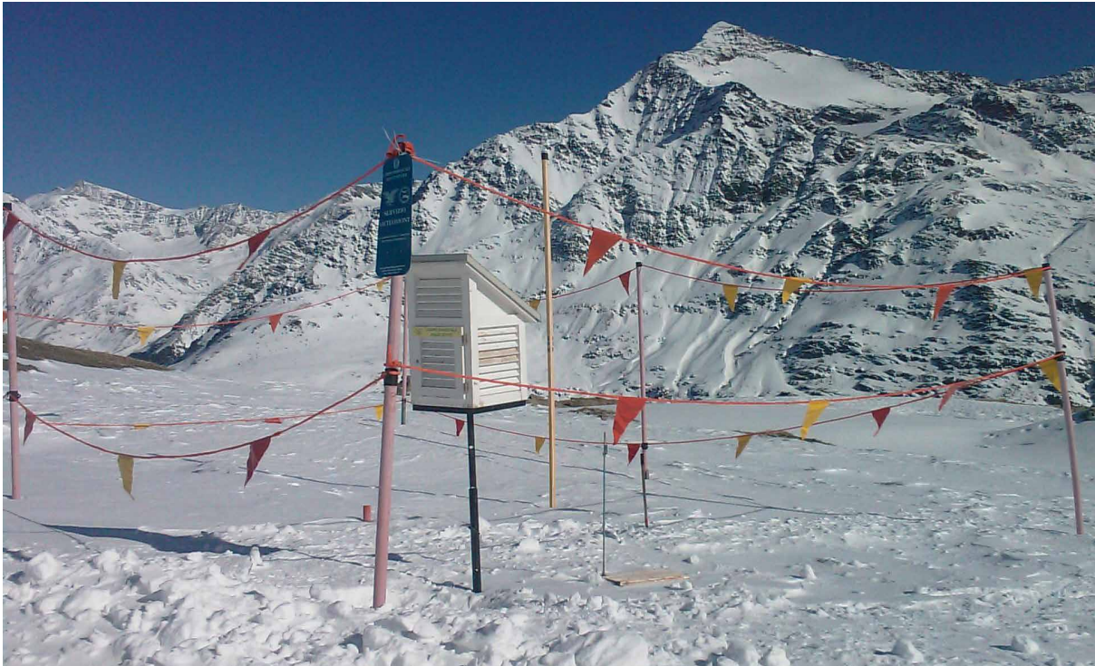
Figure I-2.19.4 Manual measurement field operated by MC, with a snow stake and a freshly placed snow board (Source: MC).
