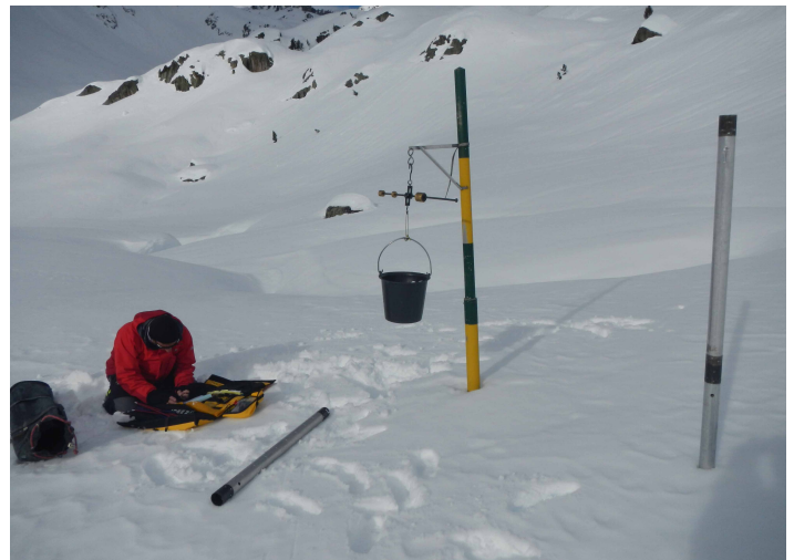
Figure I-2.13.14 Snow tube (lying on the snow) and bucket attached to a mechanical scale in order to measure the total weight of the snow (Source: EDF).
