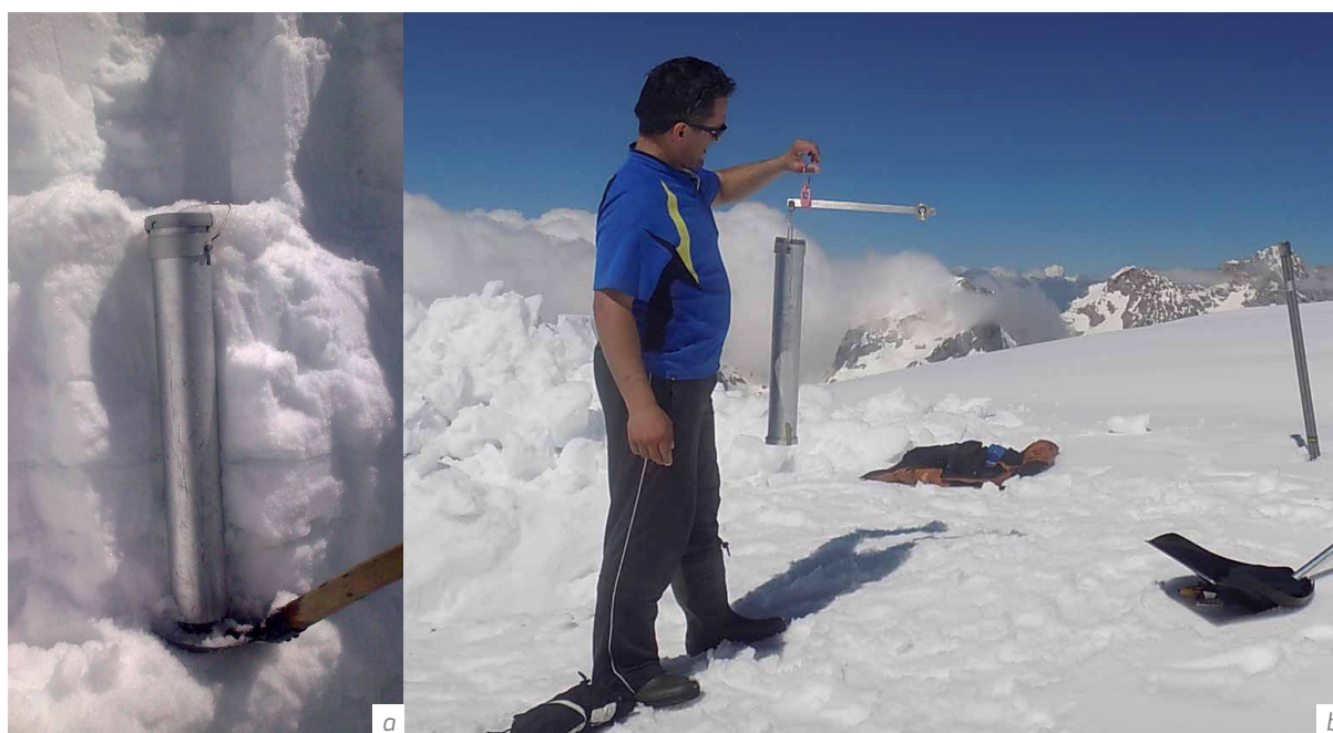
Figure I-2.33.9 Manual water equivalent of snow cover (SWE) measurements in snow pits using snow cylinders: (a) cylinder in snow pit; (b) snow cylinder attached to a steelyard balance (Source: ARSO).
