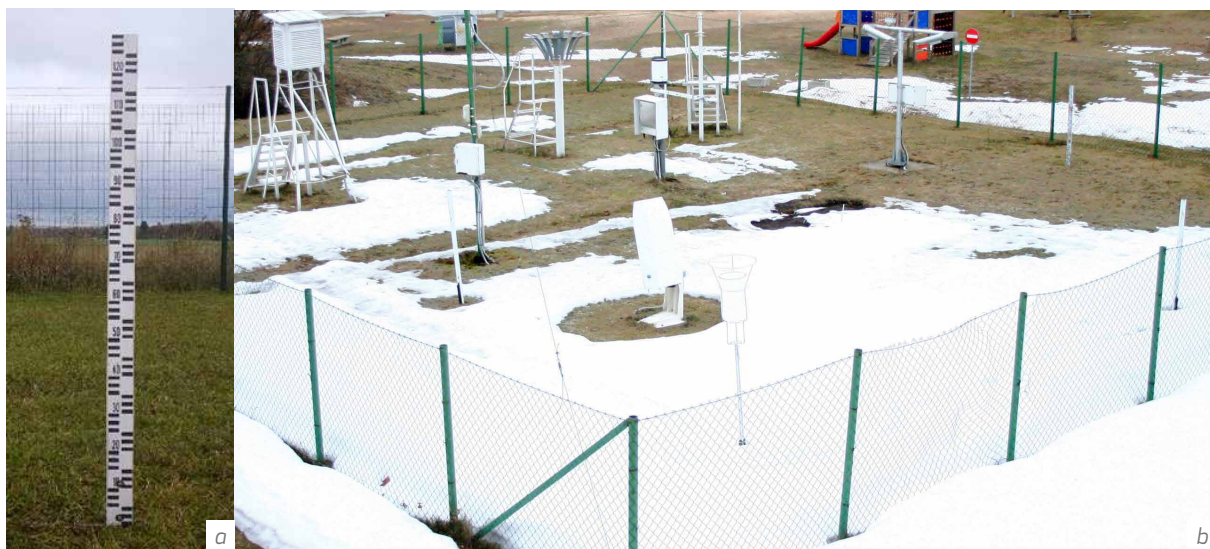
Figure I-2.11.4 (a) Fixed stake used to measure snow. (b) Snow station Narva-Jõesuu (Estonia) with three fixed stakes on 06 April 2010 (Source: ESTEA).
