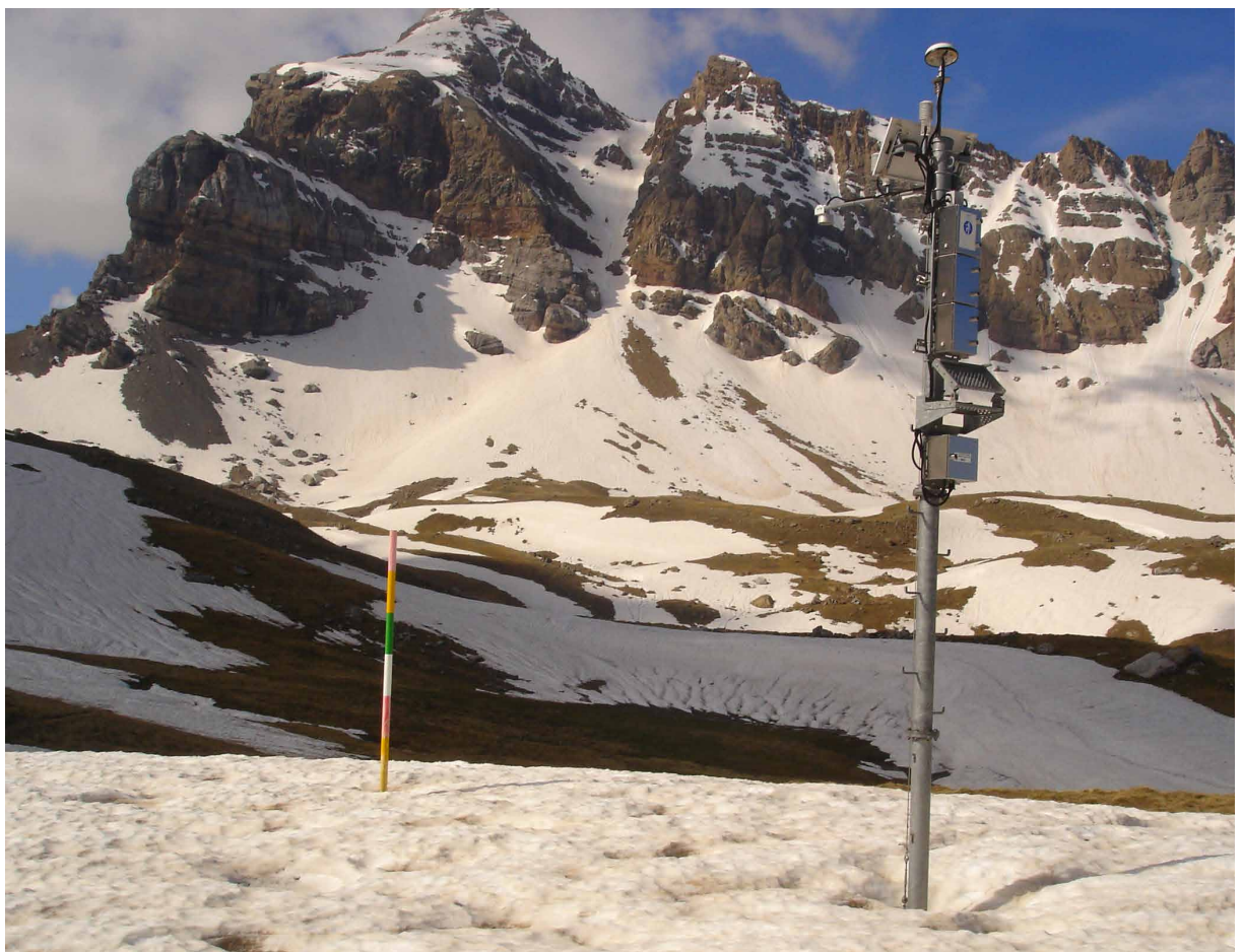
Figure I-2.34.10 Snow stake and AWS operated by GWD in Izas, Spain (Source: GWD and collaborators).
