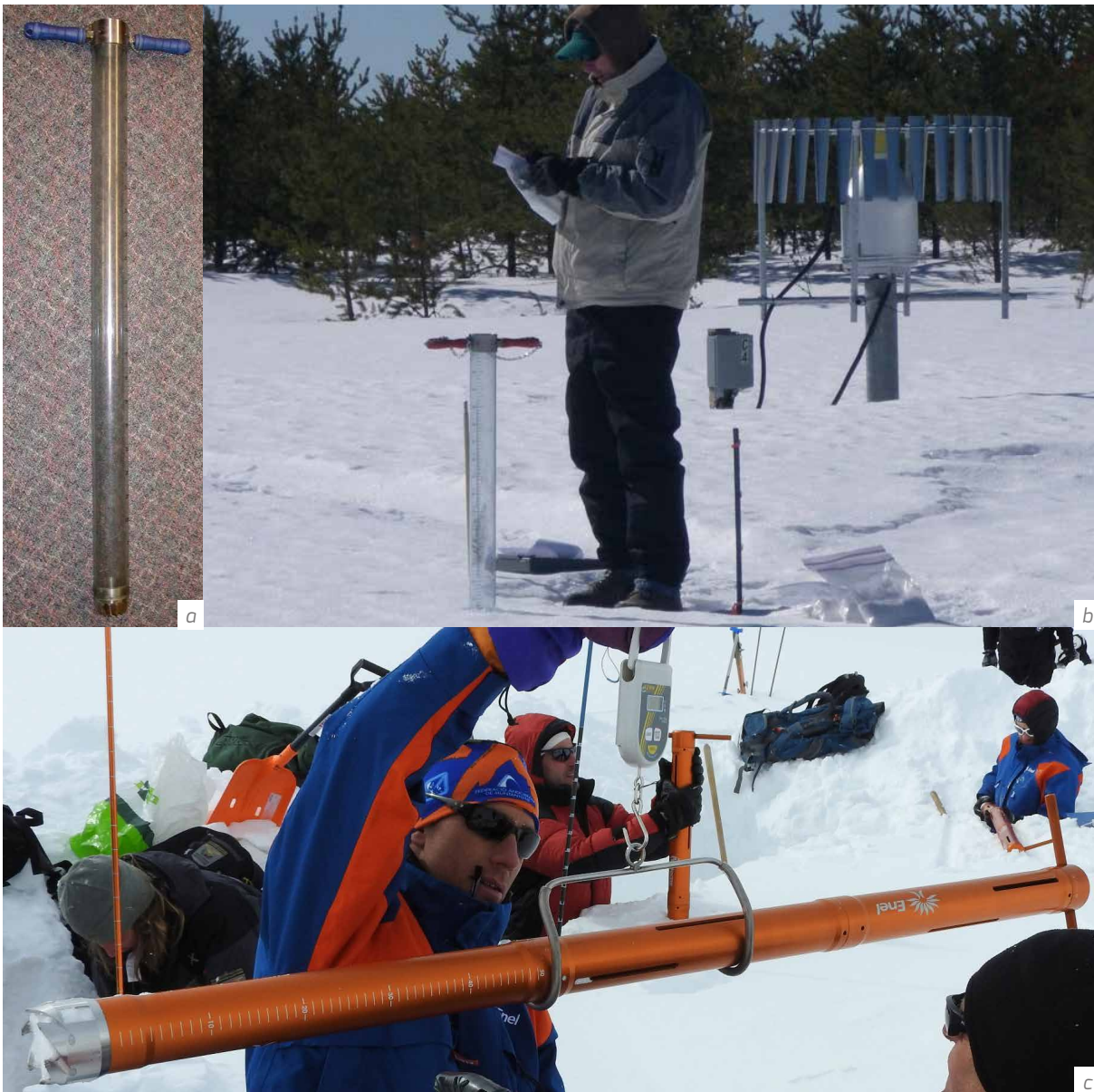
Figure I-1.5.3 Water equivalent of snow cover (SWE) measurements in snow courses using snow tubes (without snow pits): (a) snow tube (Source: ECCC); (b) SWE sampling with a snow tube (Source: ECCC); (c) snow tube placed in a snow tube cradle and attached to a scale (Source: ARPAVA).
