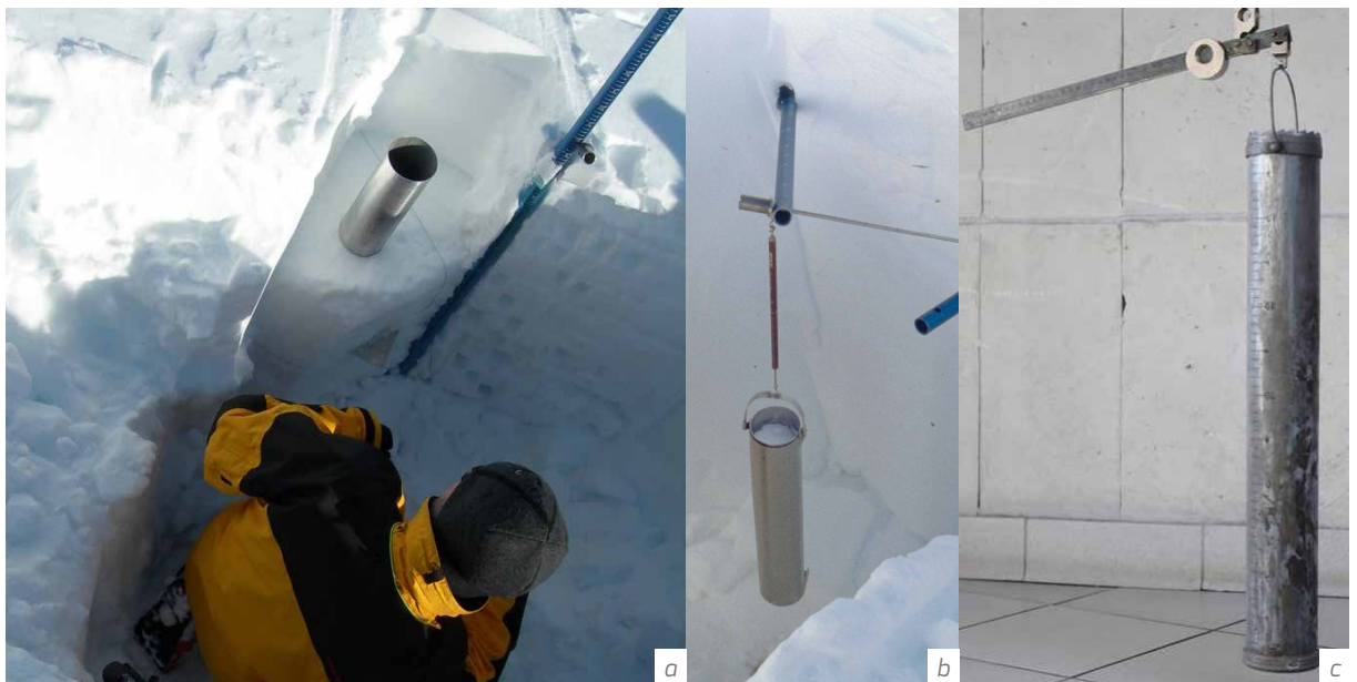
Figure I-1.5.1 Water equivalent of snow cover (SWE) measured in snow pits using a snow cylinder and scale: (a) snow sampling with a cylinder in a snow pit (Source: SLF); (b) a snow cylinder being weighed with a spring scale (Source: SLF); (c) a snow cylinder hung on a steelyard balance (Sources: ESTEA and UHMC).
