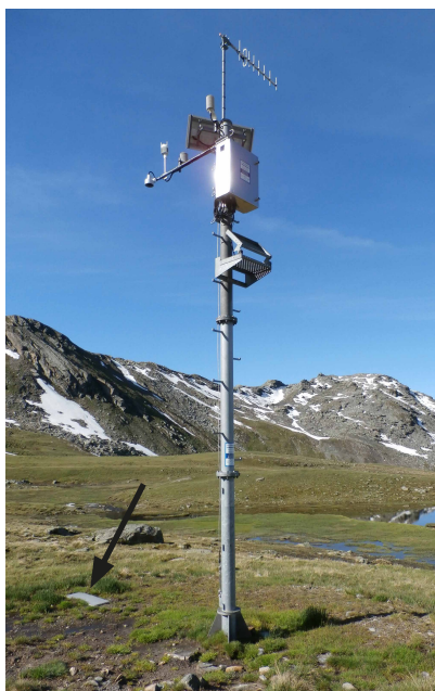
Figure I-2.13.6 Automatic weather station with a snow depth sensor, operated by EDF. To the left of the mast, a cosmic ray sensor measuring water equivalent of snow cover (SWE) automatically is visible as a white rectangular box on the ground (black arrow) (Source: EDF).
