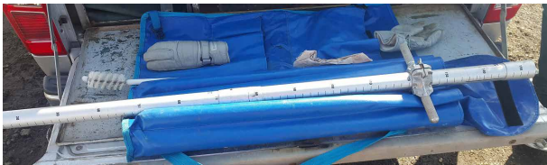
Figure I-2.37.9 Snow tube (Mt. Rose Federal) used to measure water equivalent of snow cover (SWE) manually at stations operated by TSHW (Source: TSHW).
