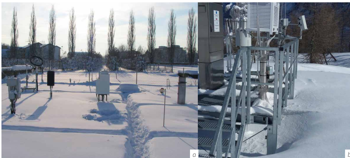
Figure I-2.33.4 (a) Fenced meteorological site in Murskasobota (Slovenia) with a fixed stake to measure snow depth manually (Source: ARSO). (b) Laser snow depth sensor at a station near the Vrsic Pass, Slovenia (Source: ARSO)
