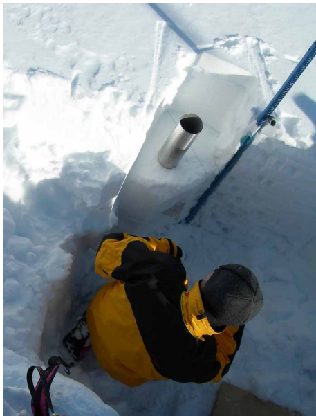
Figure I-2.36.10 Water equivalent of snow cover measurement in a snow pit; an observer is extracting snow using a snow cylinder (Source: SLF).
