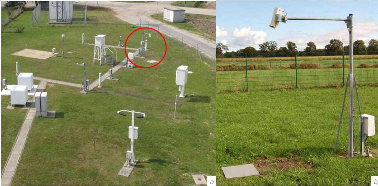
Figure I-2.14.4 (a) A DWD measurement field with a laser snow depth sensor (red circle). (b) Laser snow depth sensor SHM 30 operated by DWD with an artificial target below (Source: DWD).
