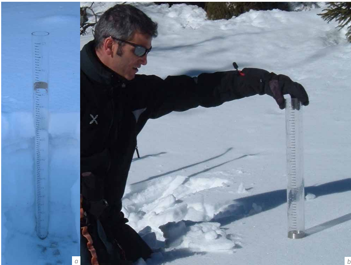
Figure I-2.19.16 (a) Plexiglas ® snow tube (developed in Italy). (b) Manual water equivalent of snow cover (SWE) measurement (without snow pit) using a Plexiglas ® snow tube, performed by ARPA Veneto (Source: ARPAV).
