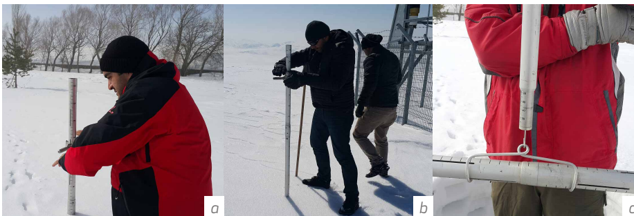
Figure I-2.37.10 (a, b) A snow sample is extracted using a snow tube at a station operated by TSHW (Source: TSHW). (c) A snow tube is placed in a snow tube cradle and attached to a spring scale in order to measure the total weight of the snow (Source: TSHW).
