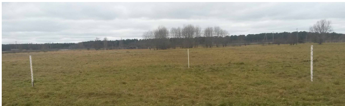
Figure I-2.20.4 A measurement field during the snow-free season, with three snow stakes arranged in a triangle for manual snow depth measurements (Source: LEGMC).
