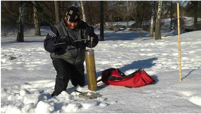
Figure I-2.12.7 Snow density measurement in a snow pit along a snow course in Finland. A wooden snow rod is visible on the far right (Source: SYKE).
