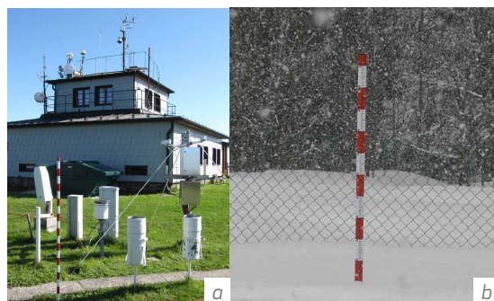
Figure I-2.9.4 Manual measurement fields with a stake to measure snow depth in (a) summer and (b) winter (Source: CHMI).
