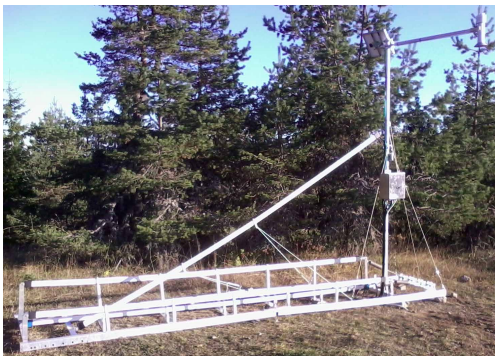
Figure I-2.6.7 Automatic station Rozhen (Bulgaria) with a Snow Pack Analyser and a USH-8 snow depth sensor (Source: NIMH).
