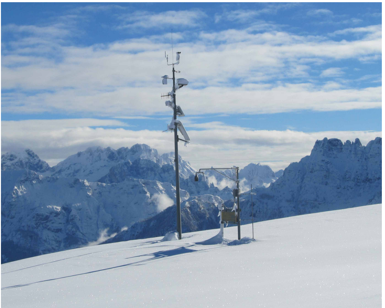
Figure I-2.19.8 Automatic weather station operated by ARPAV in Veneto, Italy, with an ultrasonic snow depth sensor (Source: ARPAV).
