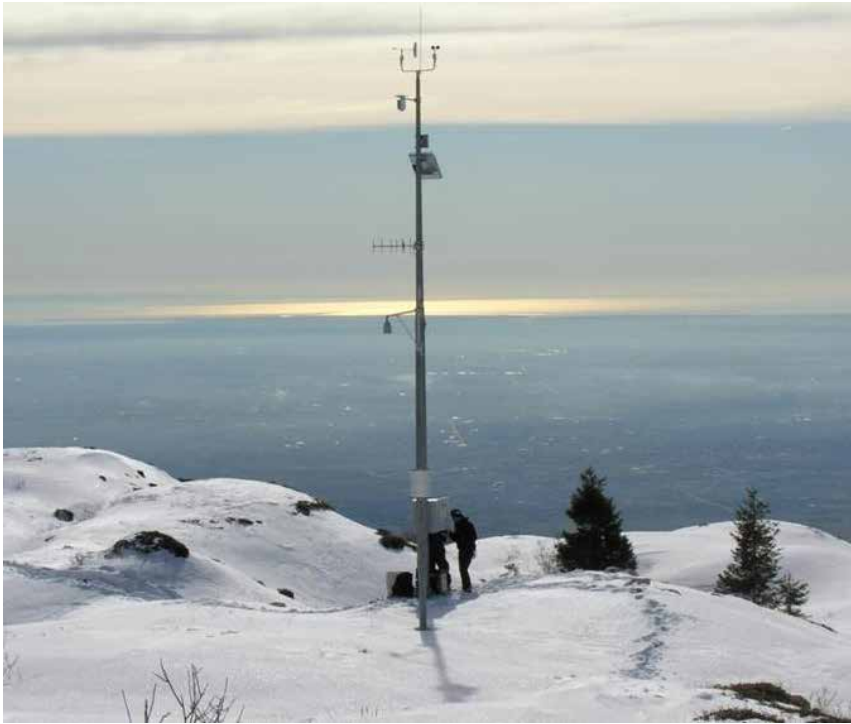
Figure I-2.19.7 Automatic weather station operated by SSCV in the region Friuli Venezia Giulia, Italy, with an ultrasonic snow depth sensor (Source: SSCV).
