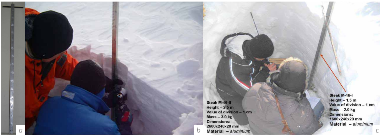
Figure I-2.38.6 (a) Portable ruler M-46 with a wooden handle. Observations in a snow pit of (b) snow characteristics and (c) snow depth using an M-46 ruler (Source: UHM).
