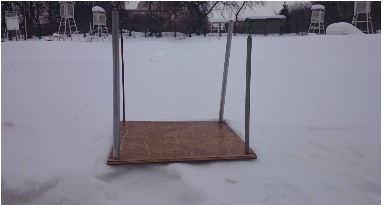
Figure I-A.7 Snow board used to measure depth of snowfall (Source: ROSHYDROMET).
