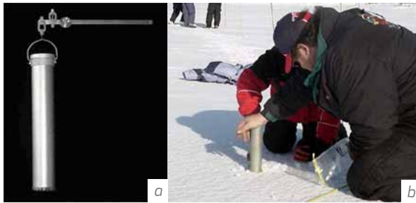
Figure I-2.20.8 (a) Iron snow cylinder attached to a steelyard balance. (b) water equivalent of snow cover (SWE) measurement along a snow course in the measurement field (Source: LEGMC).
