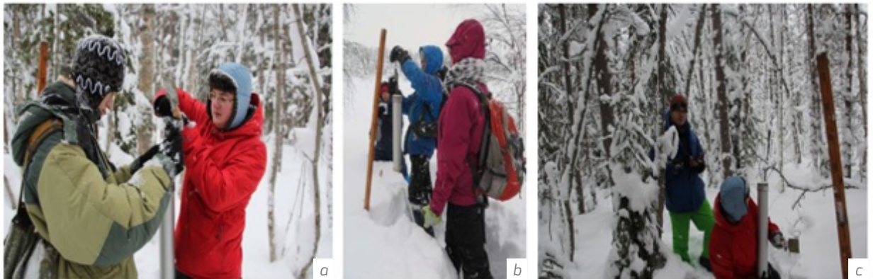
Figure I-A.11 (a-c) Water equivalent of snow cover (SWE) observations in snow pits using a snow cylinder and steelyard balance along snow courses in forested areas (Source: ROSHYDROMET).
