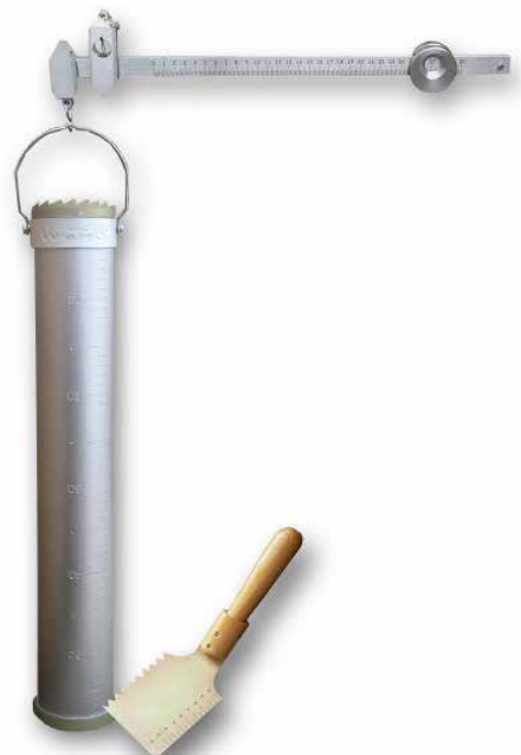
Figure I-2.14.10 Snow cylinder WS-43 attached to a steelyard balance in order to measure water equivalent of snow cover (SWE) manually (Source: DWD).
