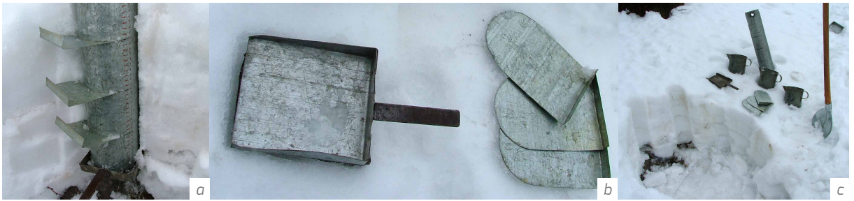
Figure I-2.7.10 (a) Hellmann cylinder; (b) snow spatula; (c) cans for melting snow (Source: DHMZ, FHMI).
