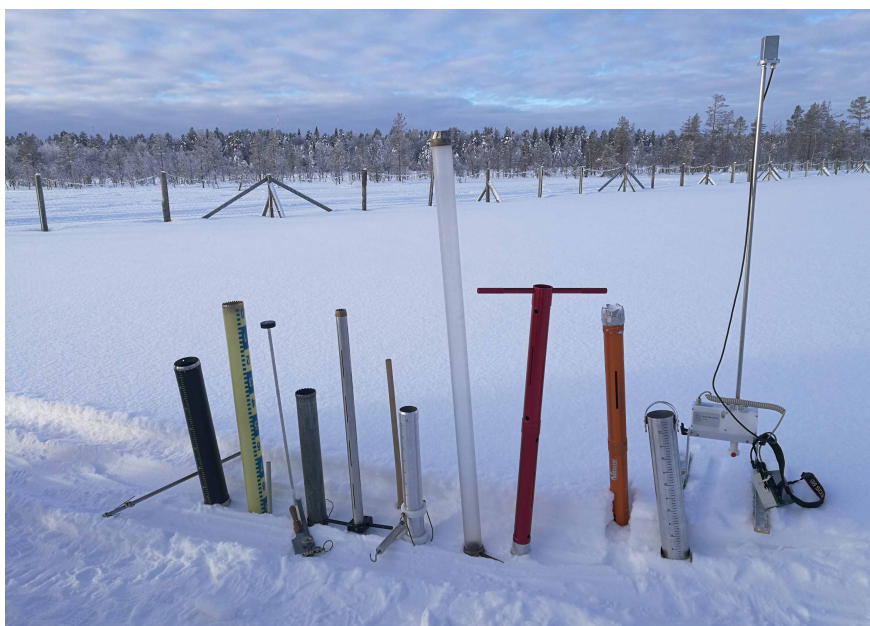
Figure II-1.2.2 Instruments used in the 3 rd HarmoSnow field campaign (from left to right): Korhonen-Melander (made and used in Finland), Dolfi (made and used in Slovakia and the Czech Republic), VS-43 (used in Estonia; made in Russia and Ukraine), U.S. Federal (used in Turkey; made in USA), IG PAS (made and used in Poland), SnowHydro (used in Spain; made in USA), Custom EV2 (made and used in Italy), Enel-Valtecne EV2 (made and used in Italy) and ETH (made and used in Switzerland). In addition, the SnowMicroPen (made in Switzerland) is shown on the far right side (Source: Cansaran Ertas).
