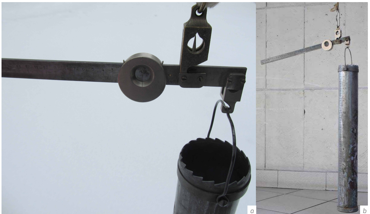
Figure I-2.11.11 Snow cylinder BC-43: (a) in weighing position; (b) attached to a steelyard balance (Source: ESTEA).
