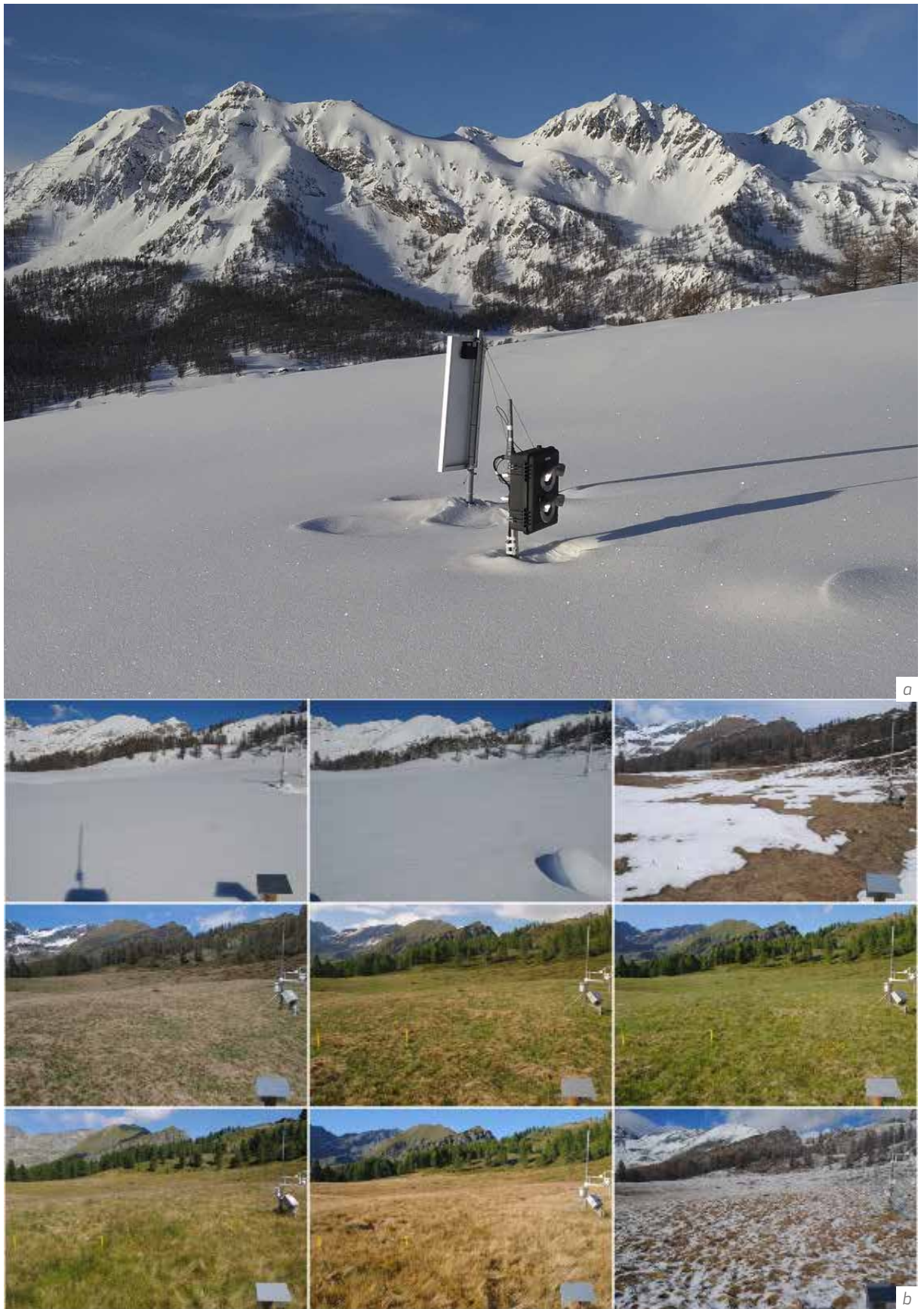
Figure I-2.19.10 (a) Webcam used to assess, among other variables, presence of snow on the ground. (b) A series of webcam images showing the evolution of the snow cover. The station in the figure is located in Torgnon-Tellinod in Valle d'Aosta, Italy and is operated by ARPAVA (Source: ARPAVA).
