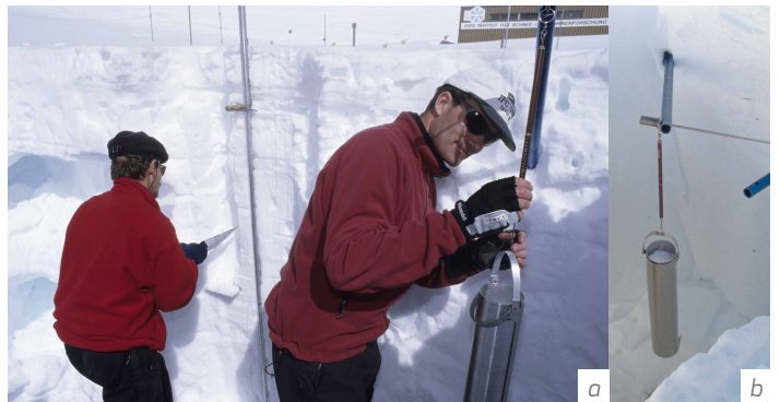
Figure I-2.36.11 (a, b) An ETH snow cylinder is attached to a spring scale during a water equivalent of snow cover measurement (Source: SLF).
