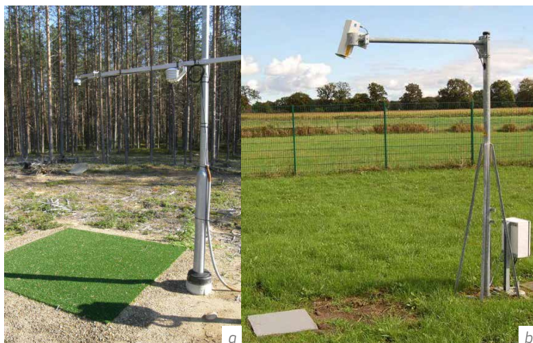
Figure I-1.2.2 Automatic snow depth instruments: (a) sonic instrument with artificial turf below (Source: FMI); (b) laser instrument with artificial target below (Source: DWD).
