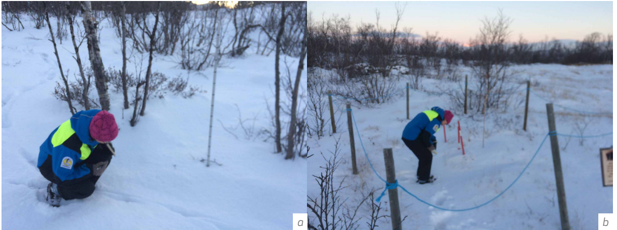
Figure I-2.35.4 Snow observations at Abisko research station in Sweden: (a) snow depth point measurement at a stake; (b) spatially distributed snow depth readings along a snow course (Source: ANS).
