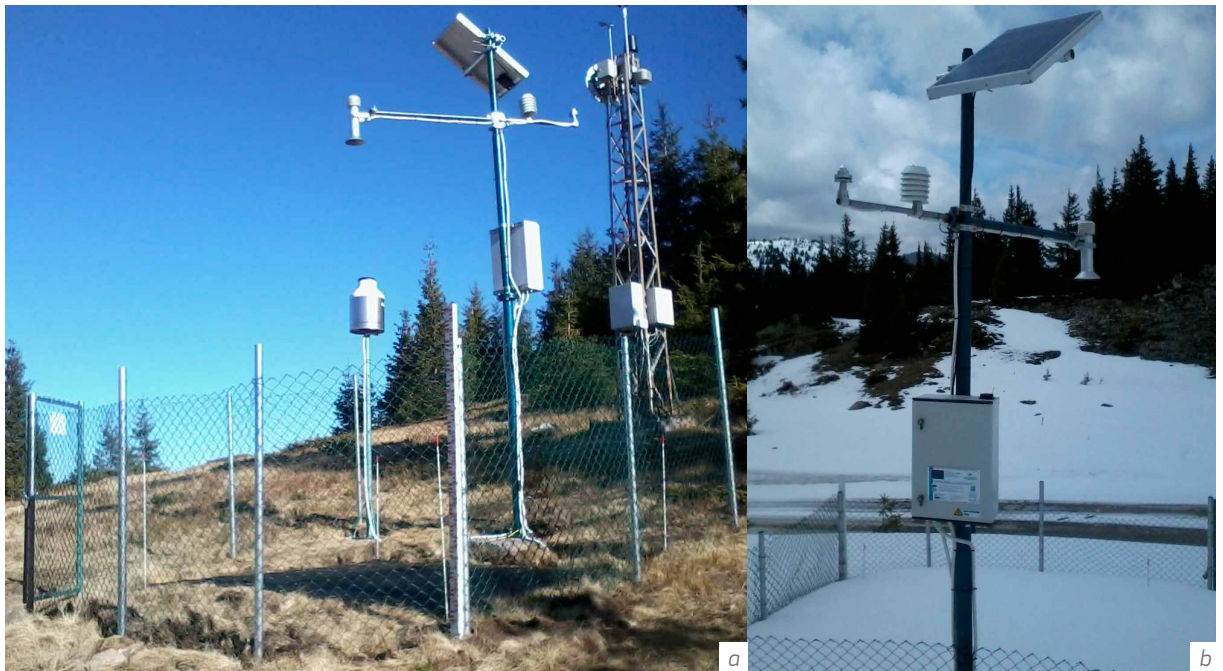
Figure I-2.6.4 Automatic weather station Perelik (Bulgaria) with USH-8 snow depth sensor during (a) the snow-free season and (b) the snow-covered season (Source: NIMH).
