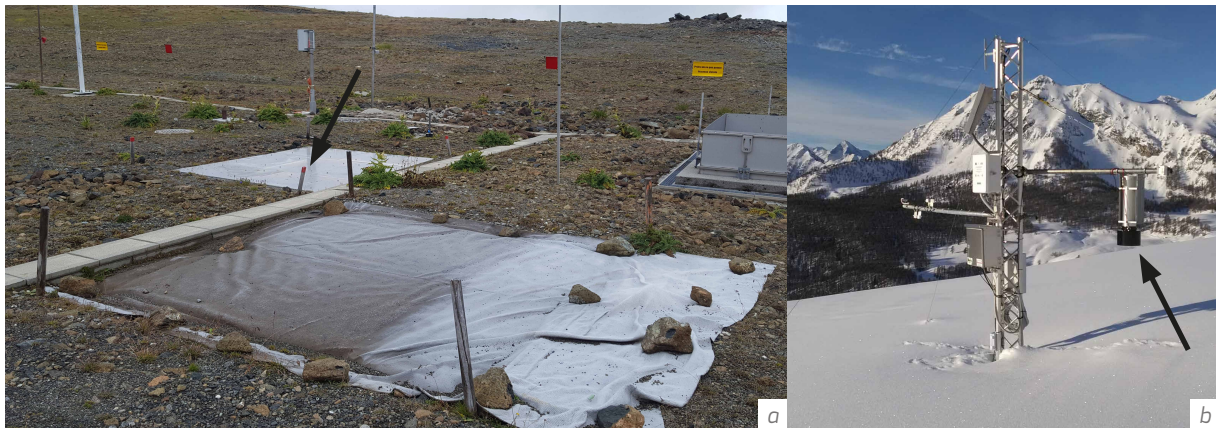
Figure I-1.5.4 Automatic water equivalent of snow cover (SWE) measurement devices: (a) snow pillow (foreground) and snow scale (background; highlighted with black arrow) at Weissfluhjoch, Grison, Switzerland (Source: SLF); (b) automatic weather station with a passive gamma radiation instrument CS725 (highlighted with black arrow) in Valle d'Aosta, Italy (Source: ARPAVA).
