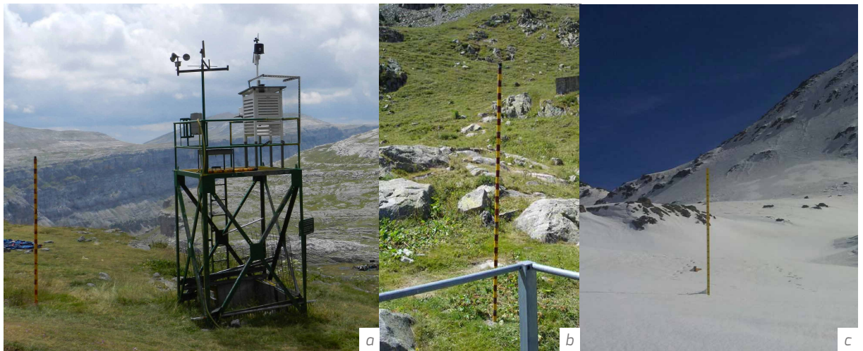
Figure I-2.34.9 Snow stakes used to manually measure snow depth at mountain stations operated by AEMET in Spain: (a) in Goriz; (b) in Angel Orus; (c) in Llauset (Source: AEMET and collaborators).
