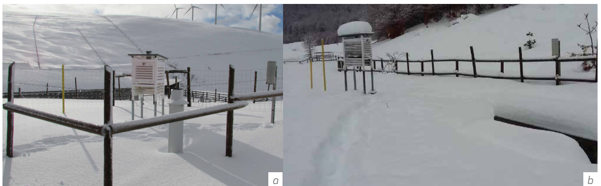
Figure I-2.34.6 Manual measurement fields with snow stakes operated by AEMET in Spain: (a) in Illano; (b) in Linza (Source: AEMET and collaborators).
