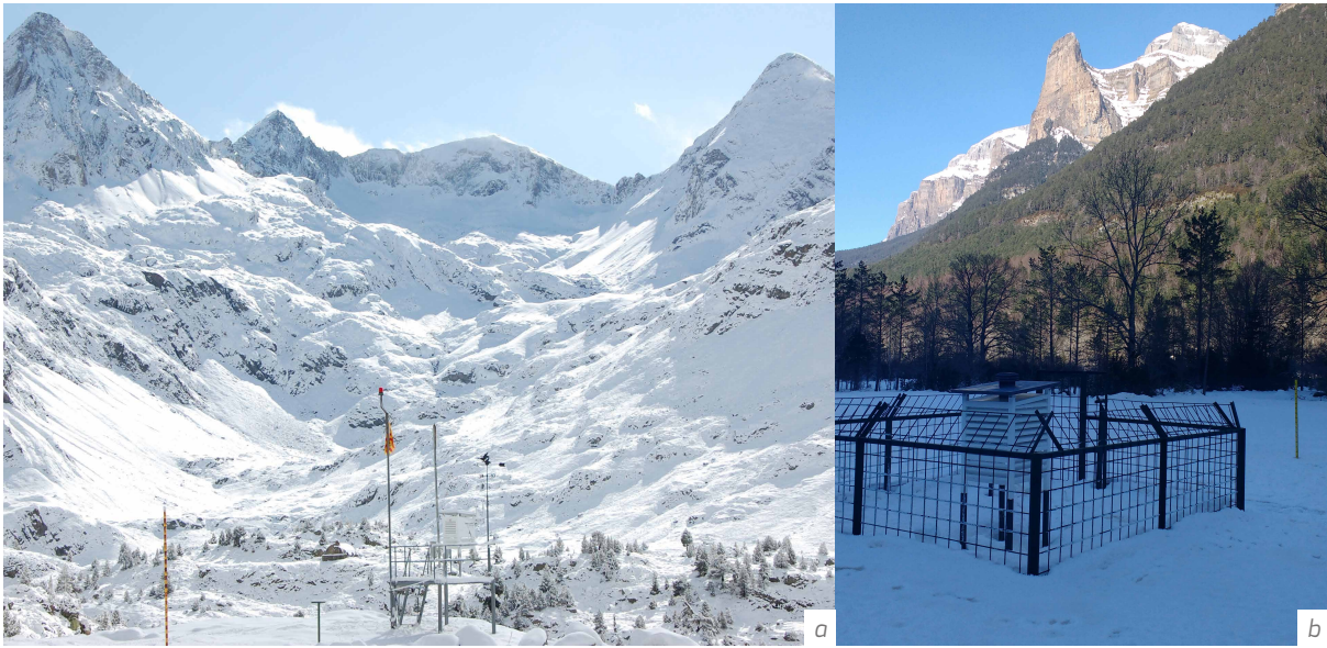
Figure I-2.34.7 Manual measurement fields with snow stakes operated by AEMET in Spain: (a) in Respomuso, Pyrenees; (b) in Ordesa National Park (Source: AEMET and collaborators).
