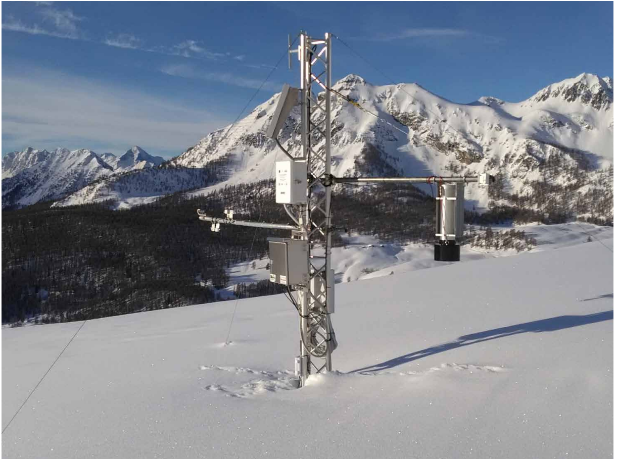
Figure I-2.19.17 Automatic weather station operated by ARPAVA in Torgnon-Tellinod in Valle d'Aosta, Italy, with a water equivalent of snow cover (SWE) gamma radiation sensor C5725 (Source: ARPAVA).
