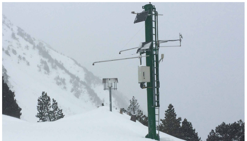
Figure I-2.2.5 Automatic snow depth measurement location in Sorteny, Andorra (Source: CENMA).
