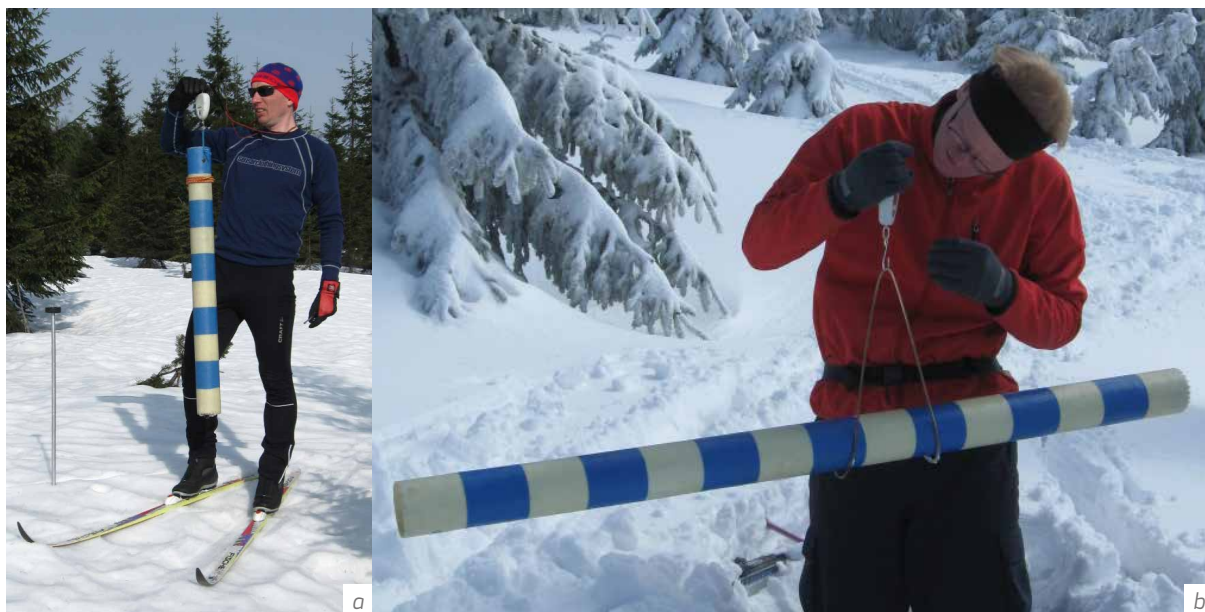
Figure I-2.9.11 Manual measurements of water equivalent of snow cover (SWE) in the Czech Republic using a laminated snow tube and a digital balance (Source: CHMI).
