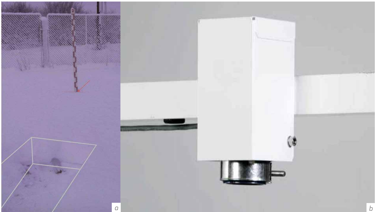
Figure I-2.30.4 (a) Example of a measurement field with a snow stake; (b) ultrasonic snow depth sensor (Source: NMA).
