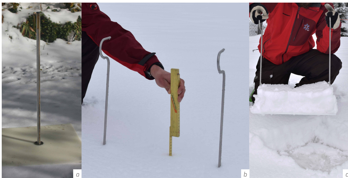
Figure I-1.4.1 Method for measuring depth of snowfall. (a) Snow board with a graduated rod attached to the centre, which doubles as a measuring device and a handle (Source: AEMET). (b, c) Depth of snowfall measured with a graduated ruler on a snow board. This board has two handles at its edges to locate the board under the snow and to assist with clearing and replacing the board after each measurement (Source: SLF).
