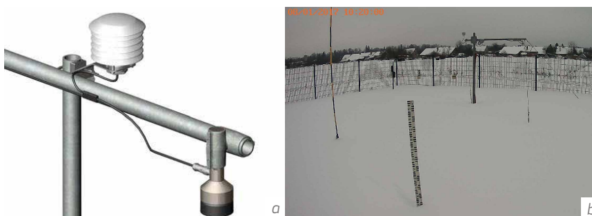
Figure I-2.20.5 (a) Ultrasonic snow depth sensor SR50AT, used at automatic weather stations (AWSs) in Latvia. (b) Webcam image of a snow stake, used to validate the automatic snow depth observations (see AWS in background) (Source: LEGMC).
