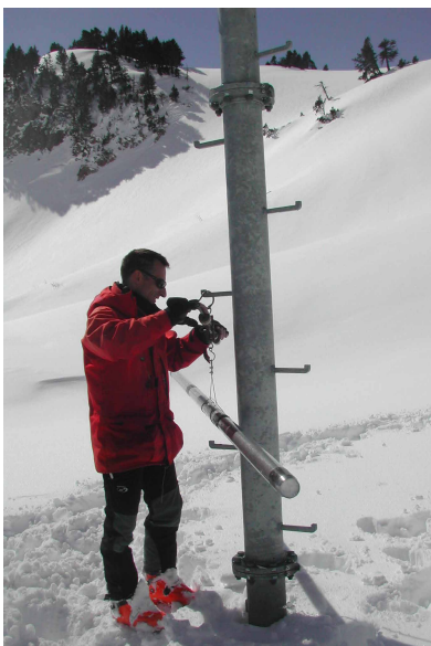
Figure I-2.13.12 Snow tube, consisting of multiple 1-m-long segments, attached to a mechanical scale at Gaougeta, France (Source: EDF).
