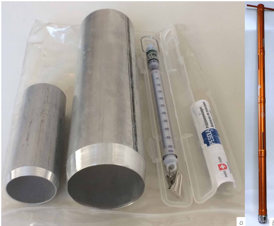
Figure I-2.19.15 (a) Snow cylinders, with volumes of 0.0001 and 0.0005 m 3 , and a spring scale (valid for a maximum weight of 0.5 kg) used to manually measure water equivalent of snow cover (SWE) in snow pits. (b) Snow tube Enel-Valtecnica (developed in Italy) used to measure SWE (Source: PAT).
