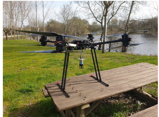
Fig. 7: Modem Payload installed
