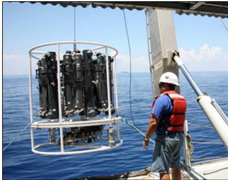
Figure 2. CTD Rosette System (CTD below sample bottles on frame) (Photo by author)
