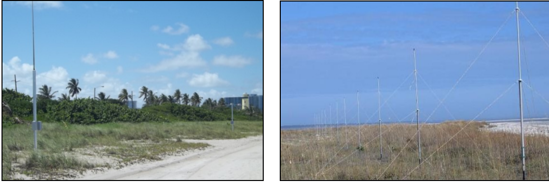
Figure 16. CODAR two-antenna (left) and WERA receive antennas (right) (Photos by author)
