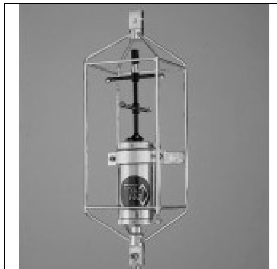
Figure 11. Acoustic Current Meter point measurement device (Gilboy et al. 1999)
