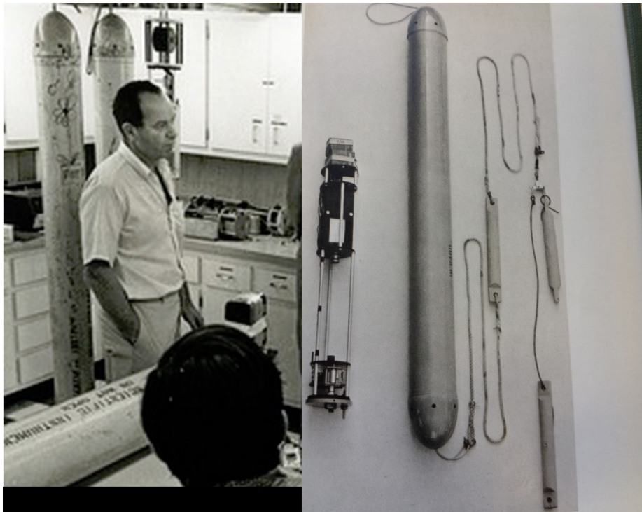
Figure 3. Dropsonde (right), and Richardson in lab with units (Photo from P. Spain)
