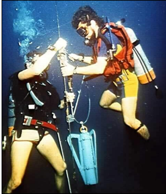
Figure 9. Niskin Wing Current Meter installed on mooring wire (University of Miami)
