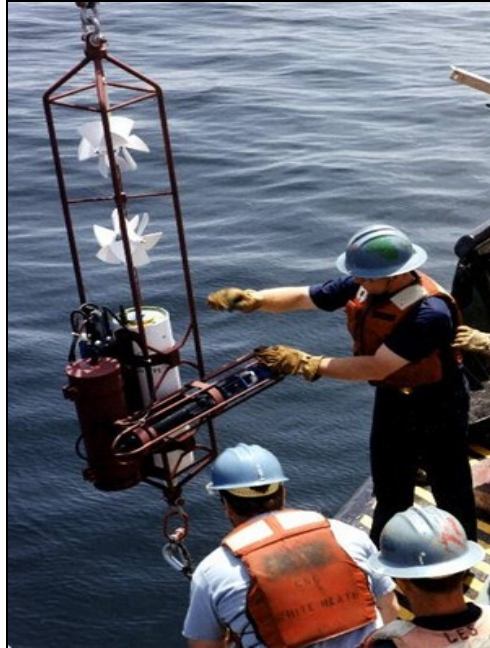
Figure 8. VMCM (note two white orthogonal rotors) (Photo by D. Blackwood WHOI)
