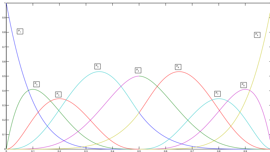
Fig. 5.5: B-spline basis function for p = 5 and C^2 .
