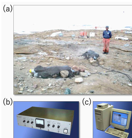
Figure 1. Picture of the ELF observation system at Syowa station. (a) Two search coil magnetometers, (b) ELF main amplifier, and (c) data recording system.
