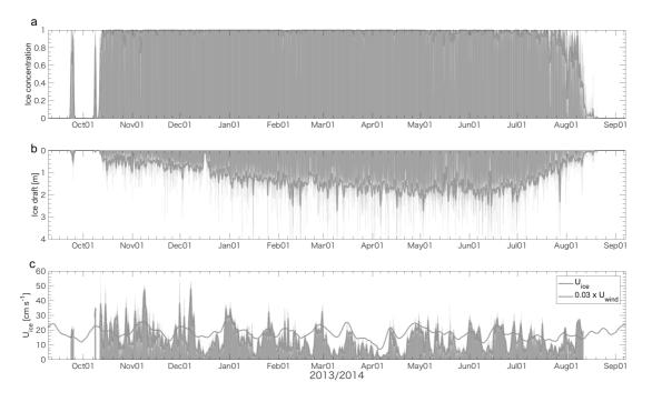
Figure: Time series of IPS-ADCP sea-ice variables: (a) sea-ice concentration (fraction: 0–1); (b) ice draft (m); (c) ice drift magnitude (cm s<sup>-1</sup>). In each plot, the raw values are 24-h running averaged.
