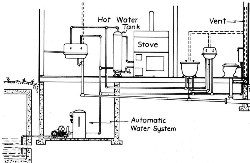
Fig. 3.—A pressure water system makes it possible to supply running hot and cold water to both the kitchen and the bathroom.
