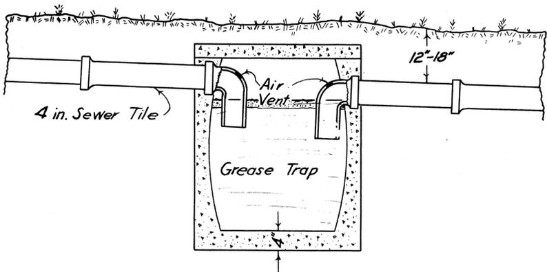
Fig. 10.—If the waste water from the sink contains very much grease, a grease trap should be installed in the drain between the sink and the septic tank.
