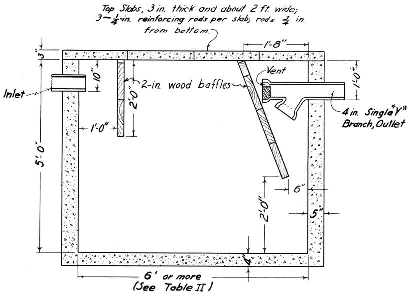
Fig. 9.—A concrete septic tank is easily constructed with home labor.
