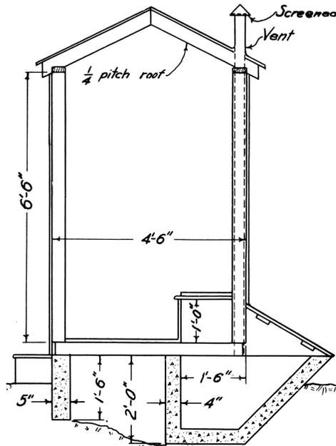
Fig. 5.—Where the soil is very open or where an earth pit privy would endanger the water supply, a water-tight concrete vault privy is recommended.
