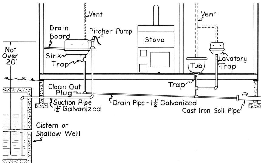
Fig. 2.—A bath tub and lavatory may be installed and connected to the sink drain.
