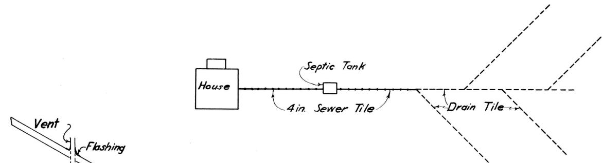
Fig. 6.—An underground tile system is usually the best method of disposal of the discharge from a septic tank.
