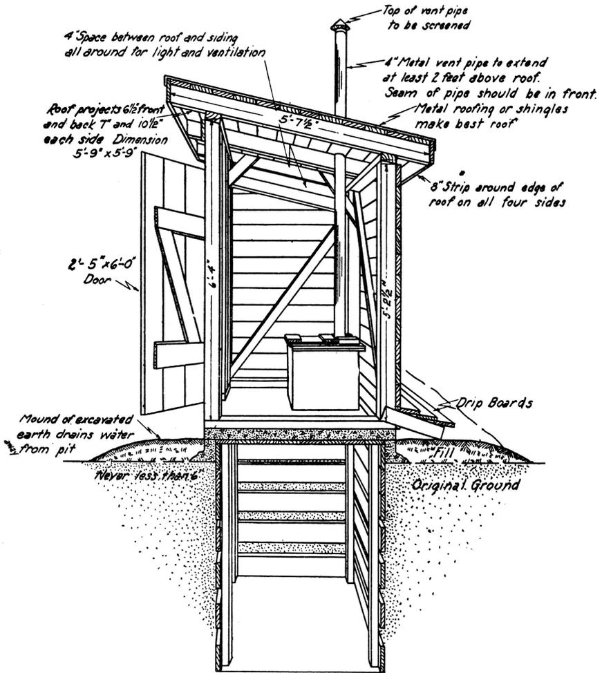
Fig. 11.—Plans of this sanitary pit privy may be secured from the State Board of Health, Jefferson City, Missouri. It is of somewhat different design and somewhat more economical to construct than the one shown in Fig. 4, page 5.
