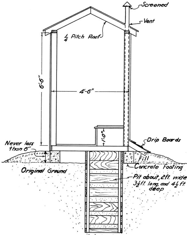
Fig. 4.—A sanitary earth pit privy provides for safe disposal of body wastes where a sewage system is not available.
