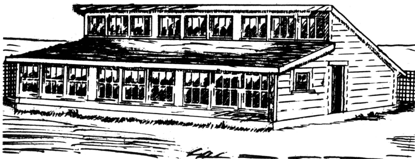
Fig. 4.—Semi-monitor house before remodeling.
