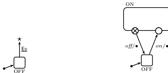
Figure 6.5: The most general model on the left and a refinement of it on the right. The right model evolves from the left one using patterns (as):ON, (a○), (a⊗), 2×(at), (ct):ON, (ct):OFF.
