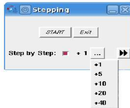
Figure 8.4: The stepping window with different actions for the forward button ((+n): jumping n steps)
