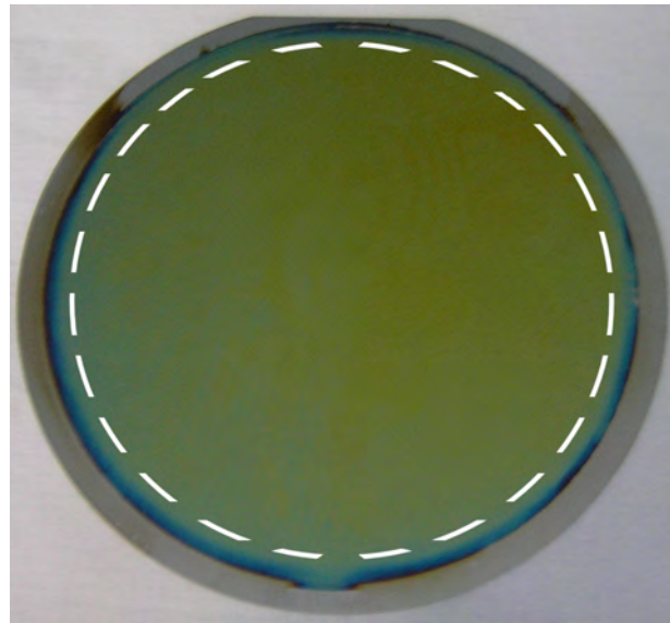
Figure 5.4: Ge wafer electrochemically etched (100) p-type Ge, HF 50% wt., j = 1 \text{ mA/cm}^2 , t = 3 \text{ h} . Note that the dashed line represents the region at which the porous layer thickness has a maximum variation of 30 nm.
