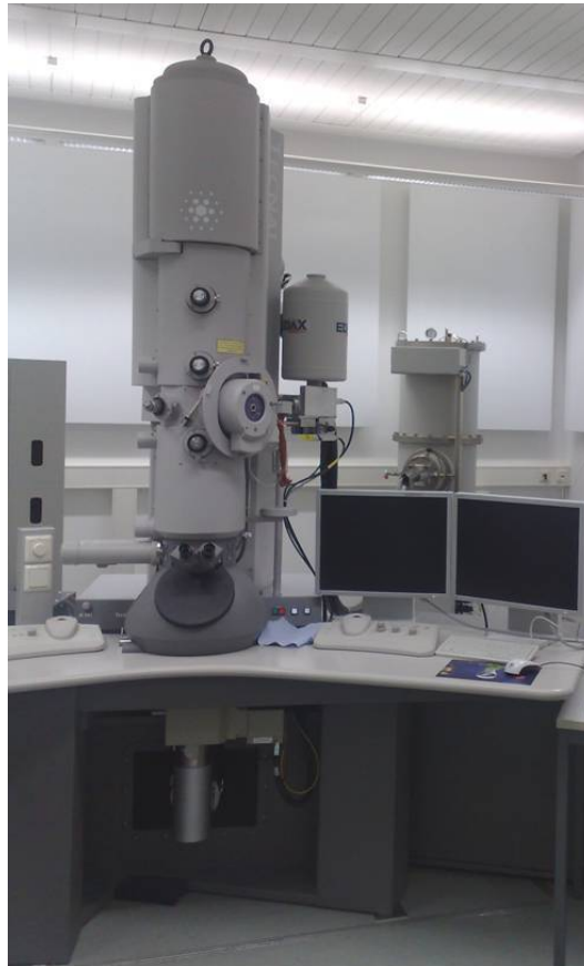
Figure 3.5: Tecnai F30G 2 (Philips) used in this thesis work.
