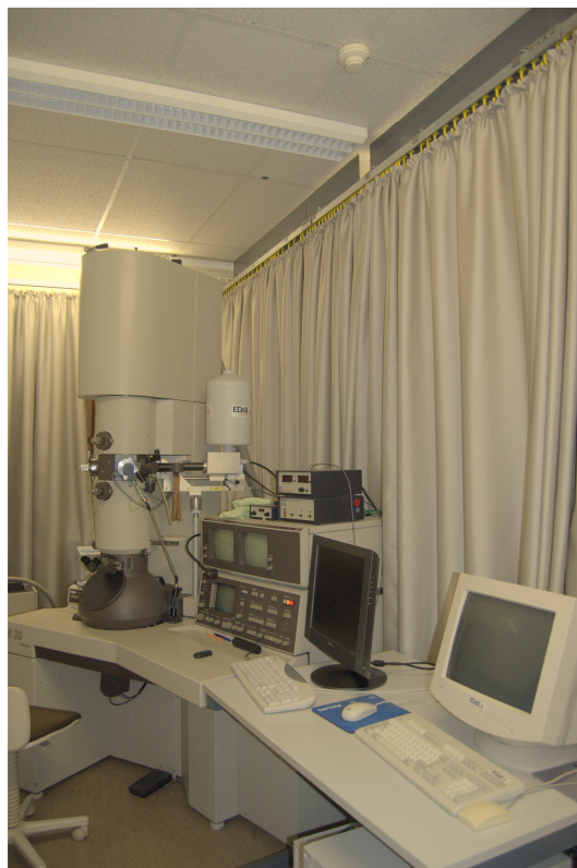
Figure 3.6: TEM CM30 used in the initial stages of this thesis work.
