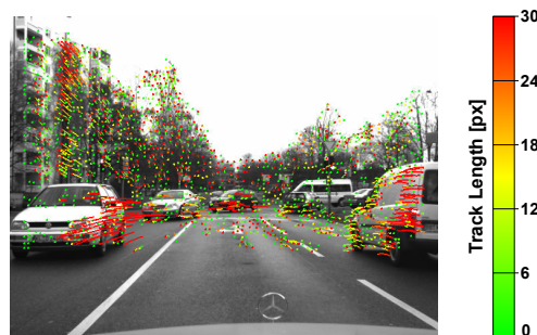
Figure 5.3: Resulting feature tracks over the last 3 frames by the spacial integration of the PowerFlow field. The color of the points indicates the age of the track: New points are green and red points indicate a track age of 5 or more frames. The color of the tracks encodes the length of the track in pixels.
