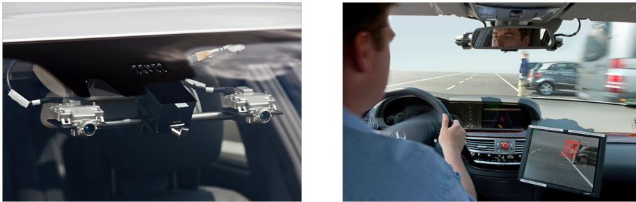
Figure 6.1: Stereo camera system installed in a Mercedes S-Class.
