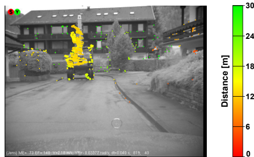
Figure 6.6: Motion field estimation result after skipping the contaminated image containing the wiper.
