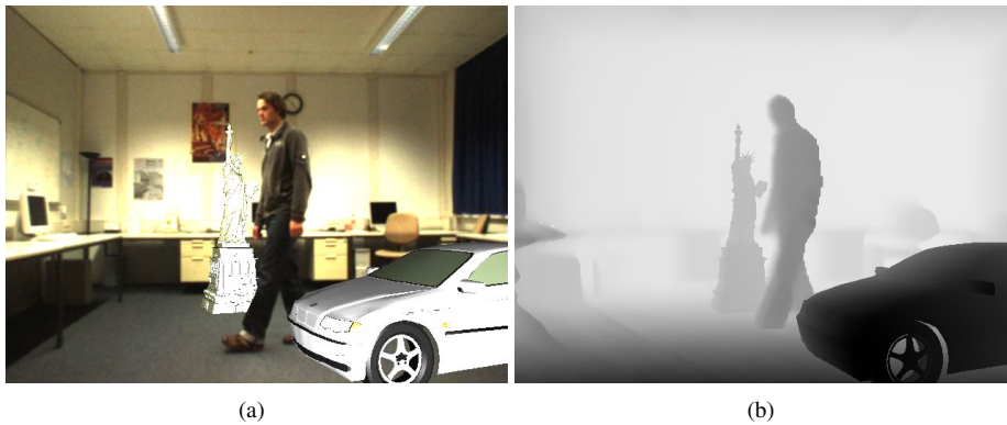
Figure 6.10.: Color- (a) and depth (b) image, composed of original images and virtual objects by depth mixing.
