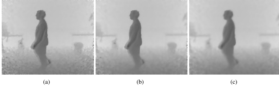
Figure 4.3.: Bilateral filtered depth images. Images have been generated with two iterations, a filter-size N, M = 3 ( 7 \times 7 ) pixel, \sigma_s = 5 and \sigma_d = 100 (a), 300 (b) and 900 (c). Observe the preserved contours of the person in comparison to mean (figure 4.1) and median filtering (figure 4.2).
