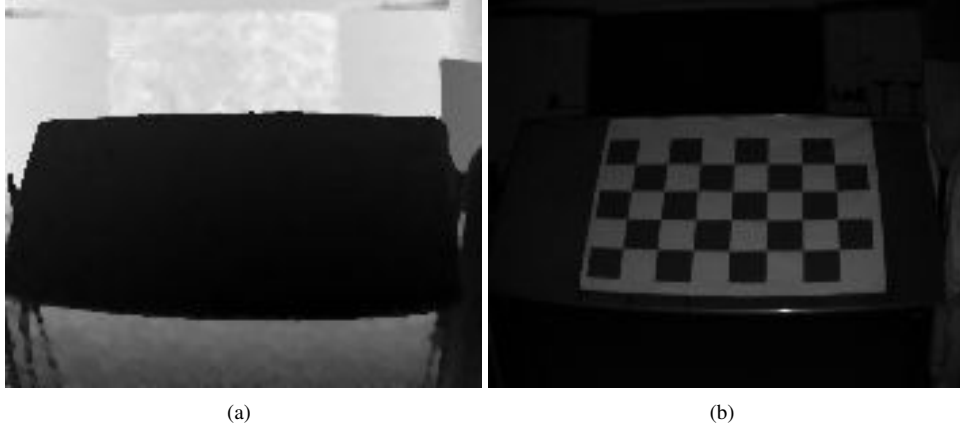
Figure 3.5.: Depth image (a) and gray value image (b) from SR4000-camera. Darker areas in (a) are closer to the camera.
