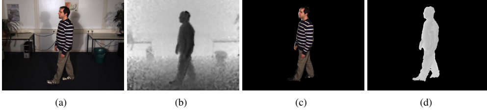
Figure 4.11.: The images of the color (a) and depth camera (b) and the segmented foreground person in color (c) and depth (d).
