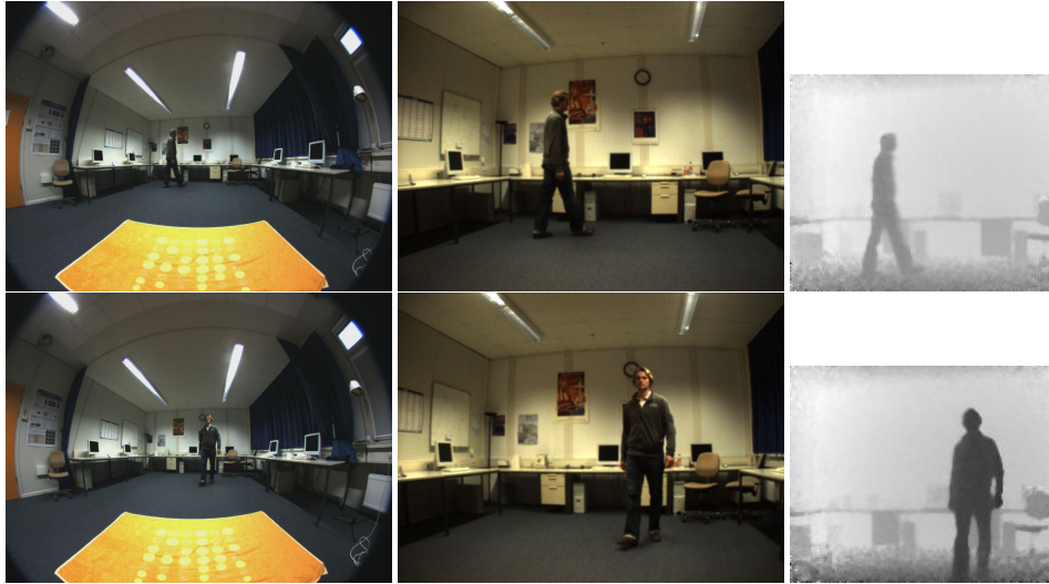
Figure 6.1.: Input images of fisheye-, target- and ToF-camera. Note that the ToF-depth images have a much lower resolution than the other images.
