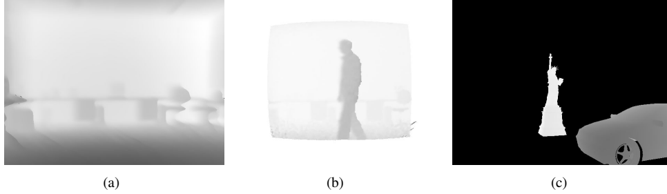
Figure 6.8.: Depth images for composition with correct occlusion handling. (a) Background depth image, (b) warped current ToF-depth image, (c) virtual depth image.
