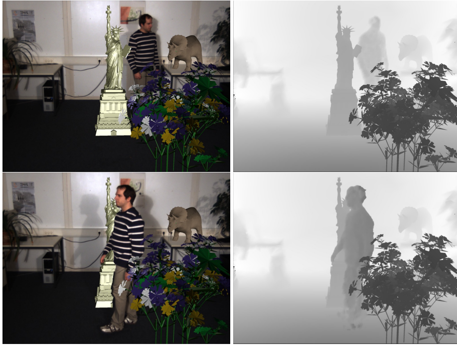
Figure 6.11.: Original image of a person, augmented by virtual objects with mutual occlusion (left). Corresponding mixed depth images (right).
