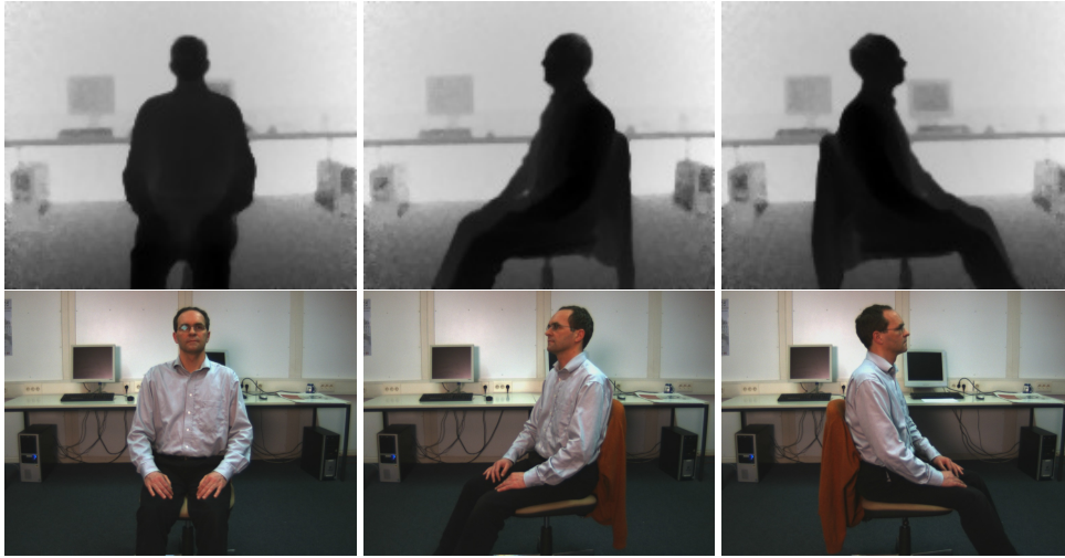
Figure 5.6.: Depth and color input images for the reconstruction of a person. Depth and color images have different resolutions ( 176 \times 144 pixel and 1024 \times 768 pixel).
