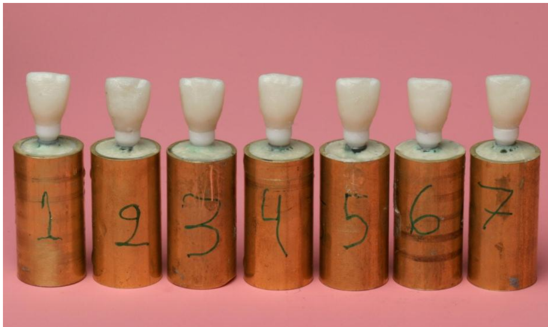
Figure 3.4. Typical group after completion of the bonding procedure.
