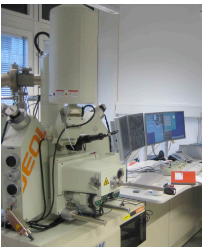
Figure 14: Picture of the electron microprobe used for volcanic glass composition determination at the east-shore campus of IFM-GEOMAR.
