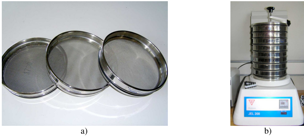
Figure 1.2 Set of sieves – a) and mechanical shaker –b) used for sieving analysis
