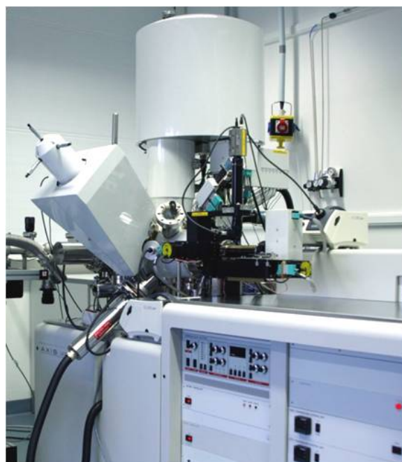
Figure 3.12: Photograph showing the XPS machine used to analyse the Co–pp HDMSN nanocomposites.
