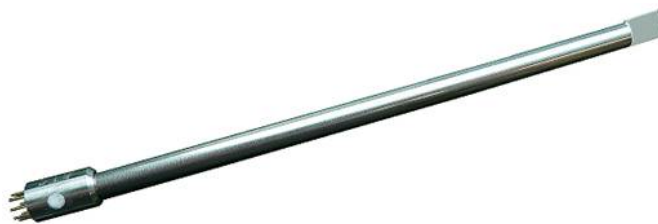
Figure 3.4: Photograph of the active thermal probe used to measure the energy influx in the sputtering chamber [73].
