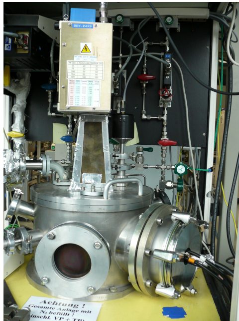
Figure 3.3: Photograph of sputtering reactor used to prepare cobalt–plasma polymerized HMDSN nanocomposites.
