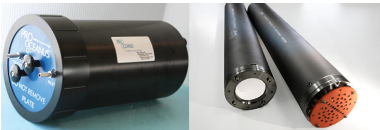
Figure 2.2 Left: The PSI \text{CO}_2 -Pro sensor with a diameter of 19 cm and a length of 49 cm. The sensor features a tubular membrane interface with an in- and outlet on the front cap. Right: Two HydroC sensors with a planar membrane interface. The housing has a diameter of 9 cm and a length of 38 cm.
