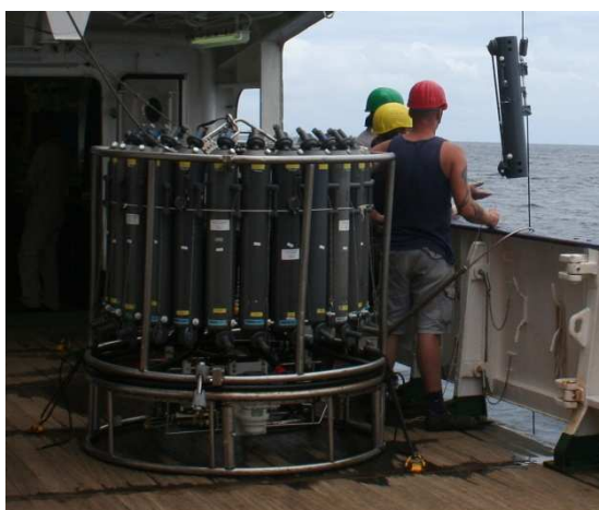
Fig. 4.1: In the left corner the CTD rosette and on the Kevlar rope a GoFlo bottle attached coming out of the water (Foto: M. Dunker).
