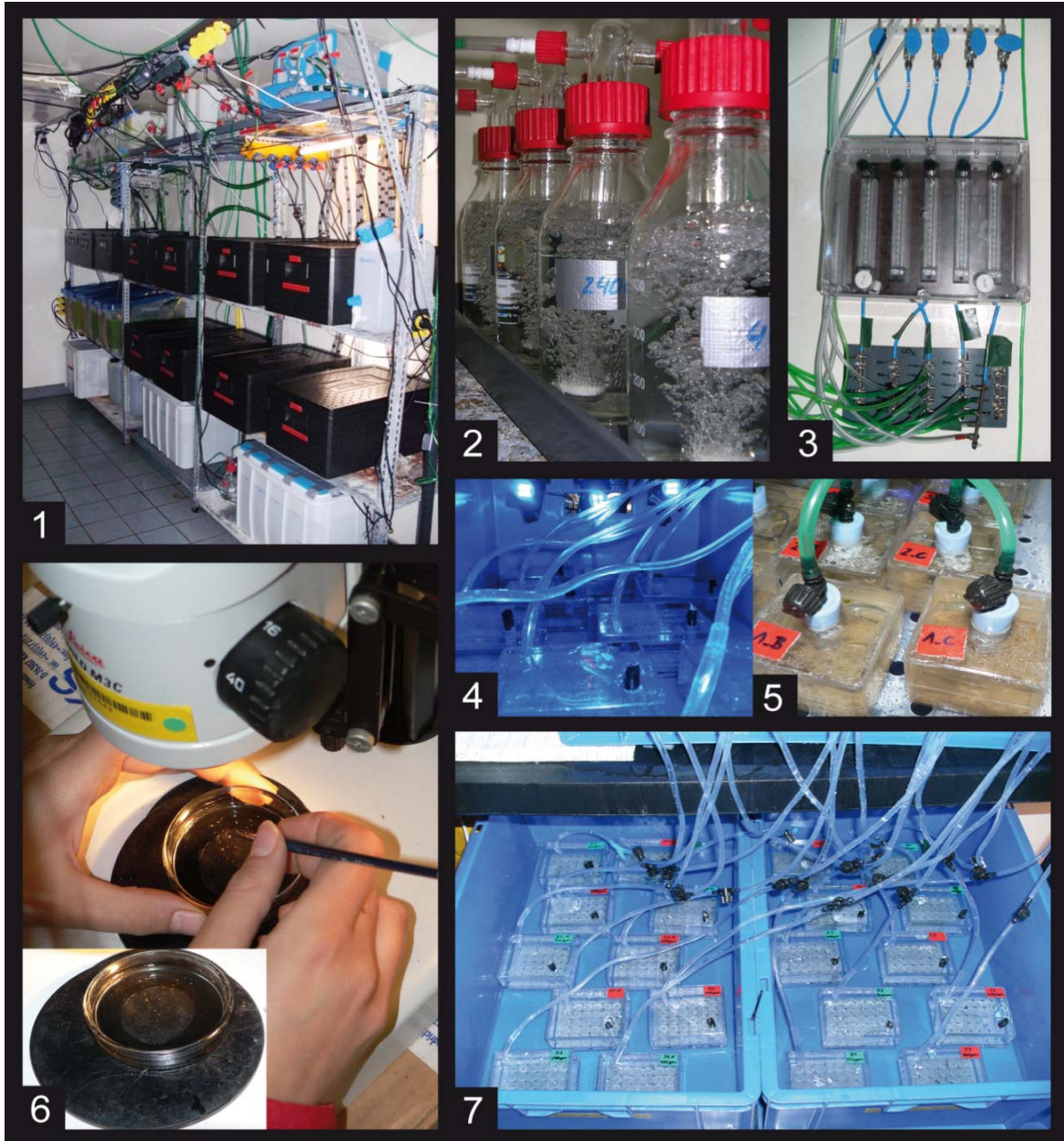
Fig. II.3: Experimental design: 1) experimental set up, 2) gas-washing bottle, 3) valves of the CO 2 gas-flow regulation unit, 4) water tubes, 5) taps regulated water flow, 6) picking of foraminifera and 7) culture vessels with recruitment pits .
