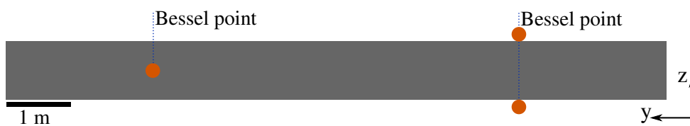
Figure 5.11: Mounting schema for the granite substructure. The positions of the setup points are marked with the orange circles. The orientation is defined because of mounting the structure in three points only. To minimize bending of the granite, the points are placed in the Bessel distances of the long axis.
