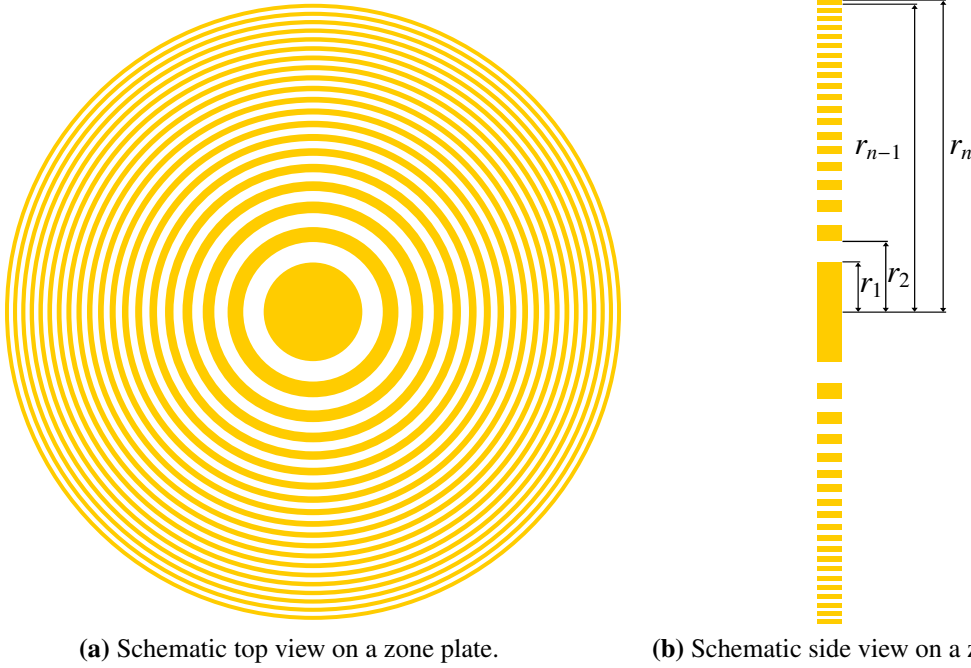
Figure 2.12: Sketch of a zone plate. The radii for the different orders are marked in (b).
