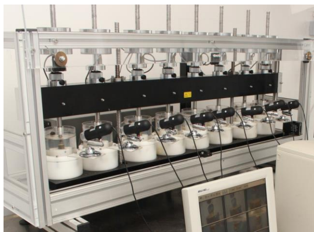
Fig. 16: Multifunction chewing simulator (Willytec)
