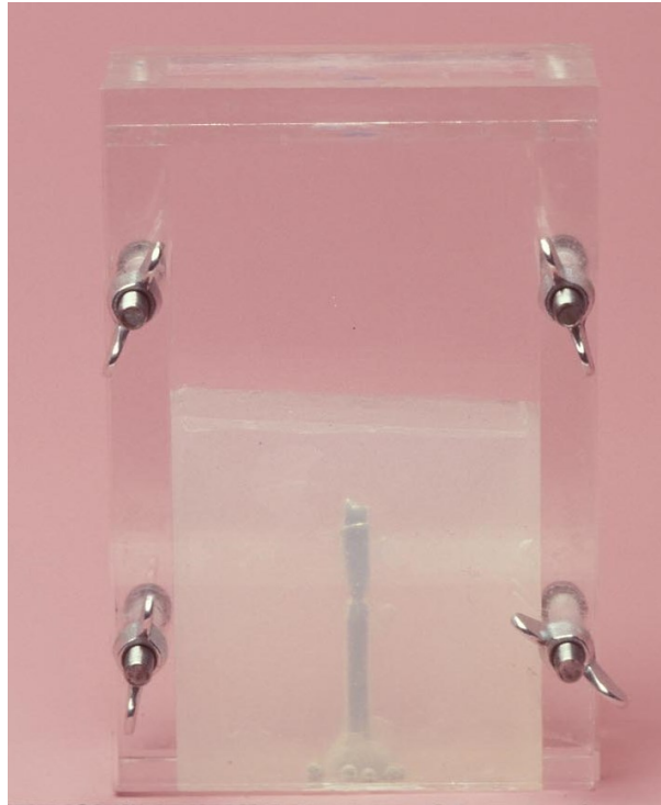
Fig. 3. Duplicated mold was poured by melting speedy wax.
