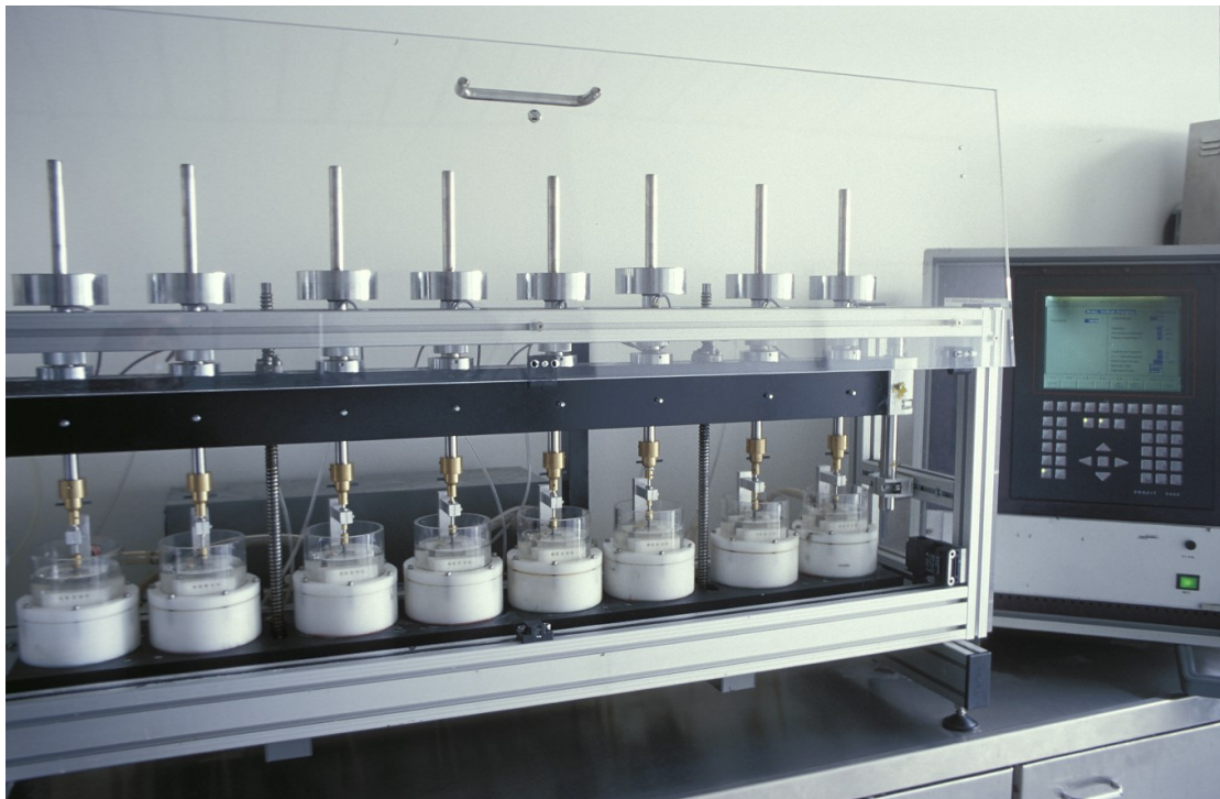
Fig. 11. Clasps within DRHDs were mounted in the chewing simulator device.
