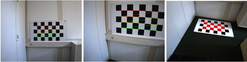
Figure 4.2. Images of a checkerboard pattern for intrinsic camera calibration captured from different view points and at different positions with detected corners drawn into. The right image is overlaid with a rendering of the checkerboard.
