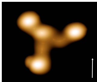
Figure 7.6: Constant current images of ReA trimer on Au(111). Scale bar indicates 1 nm and a \langle 1\bar{1}0 \rangle direction.
