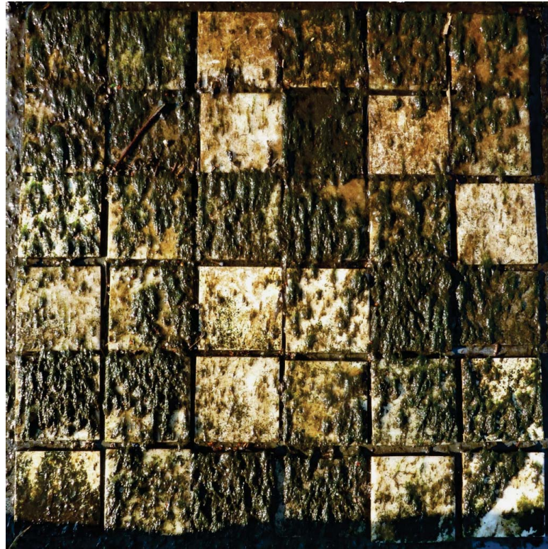
Figure 65: Fouled PTU/silicone-composites after 12 months of immersion in the river Schwentine. PTU and AlMg3 are shown as references. The sample surfaces with reduced fouling belong to PTU/ETAS composites with additional ZnO particles of both morphologies and concentrations. The sample size amounts to 80 mm * 80 mm.
