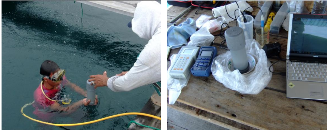
Fig. 2-11 Diver with sediment sample in PVC tube (left). Samples were analysed with Probes immediately after the sample was obtained (right) (Photos: K.-H. Runte 2015)
