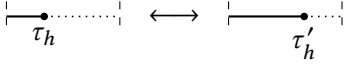
Figure 3.15: Move the head of the worm in imaginary time. This simple MC step is essential for the sampling of the MGF.
