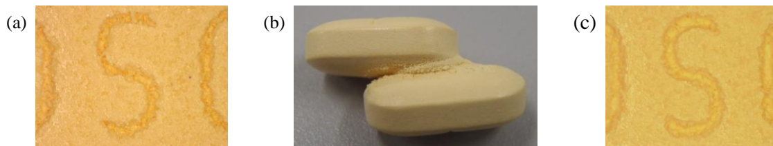
Figure 3 Appearance of film coated tablets: (a) appearance of the deboss in the conventional process parameter setting procedure (b) twinning observed in the conventional process parameter setting procedure (c) appearance of deboss in the proposed process parameter setting procedure
