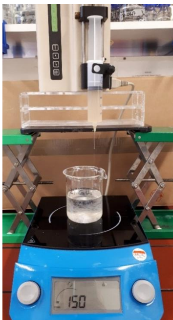
Figure 7.1: Picture of the pectin bead preparation technique used in the present study
