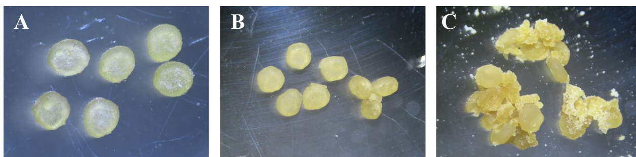
Figure 7.16: Effect of ethanolic shellac coating for 60 min (A), wd-shellac coating for 1 min (B) and wd-shellac coating for 5 min (C) on morphology of P5.9 hydrogel beads (two-step-procedure) after drying. Light microscope pictures; 20 times magnification (A); 10 times magnification (B, C).
