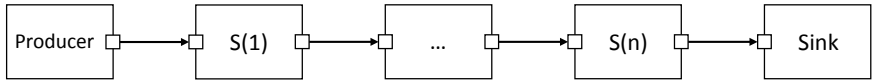
Figure 13.1. Pipeline configuration used as micro-benchmark for the overhead evaluation of TeeTime’s unsynchronized pipe.
