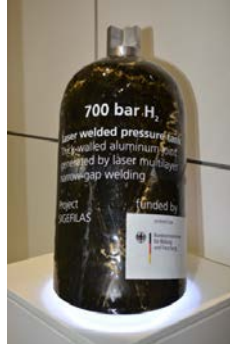
Figure 8: Prototype of a 700bar car H 2 pressure tank with laser welded connection (welding depth 25mm)
