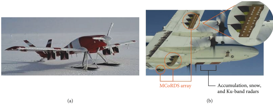
FIGURE 1: Meridian UAS with four Vivaldi antennas integrated below wing [16] (a) and NASA P-3 with all sensors installed [9] (b).
