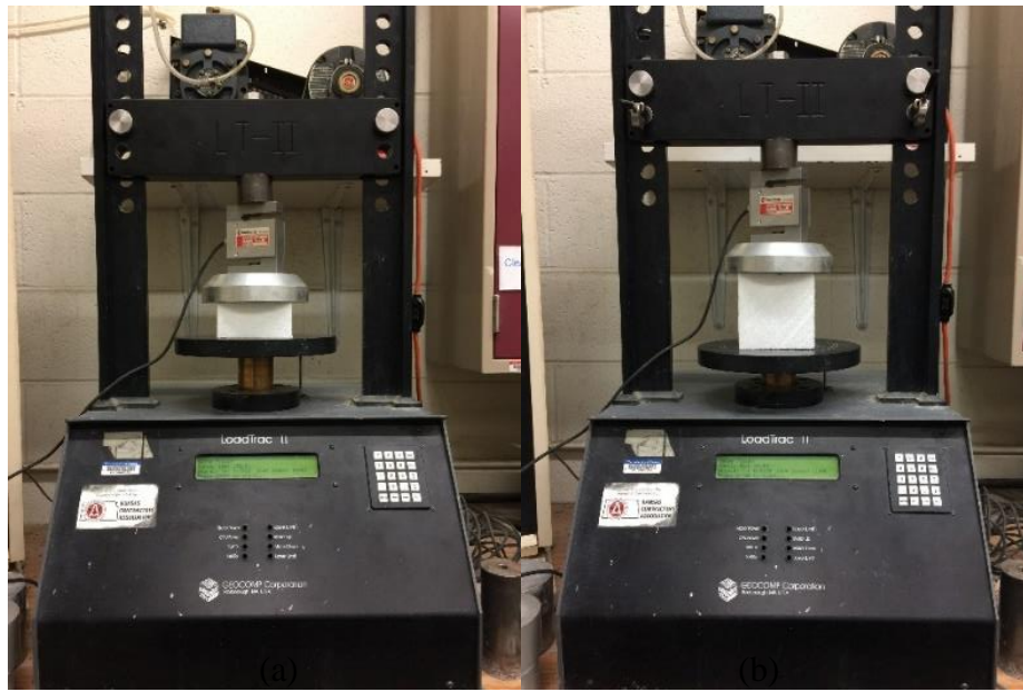
Figure 4.9 Test setup for the isolated EPS geofabric with a thickness of (a) t = 50 mm; and (b) 2t = 100 mm.
