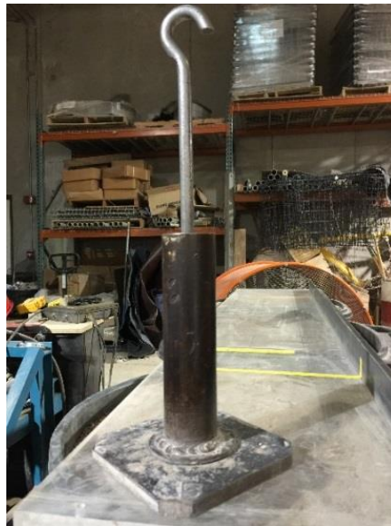
Figure 3.3 Manual steel compactor.
