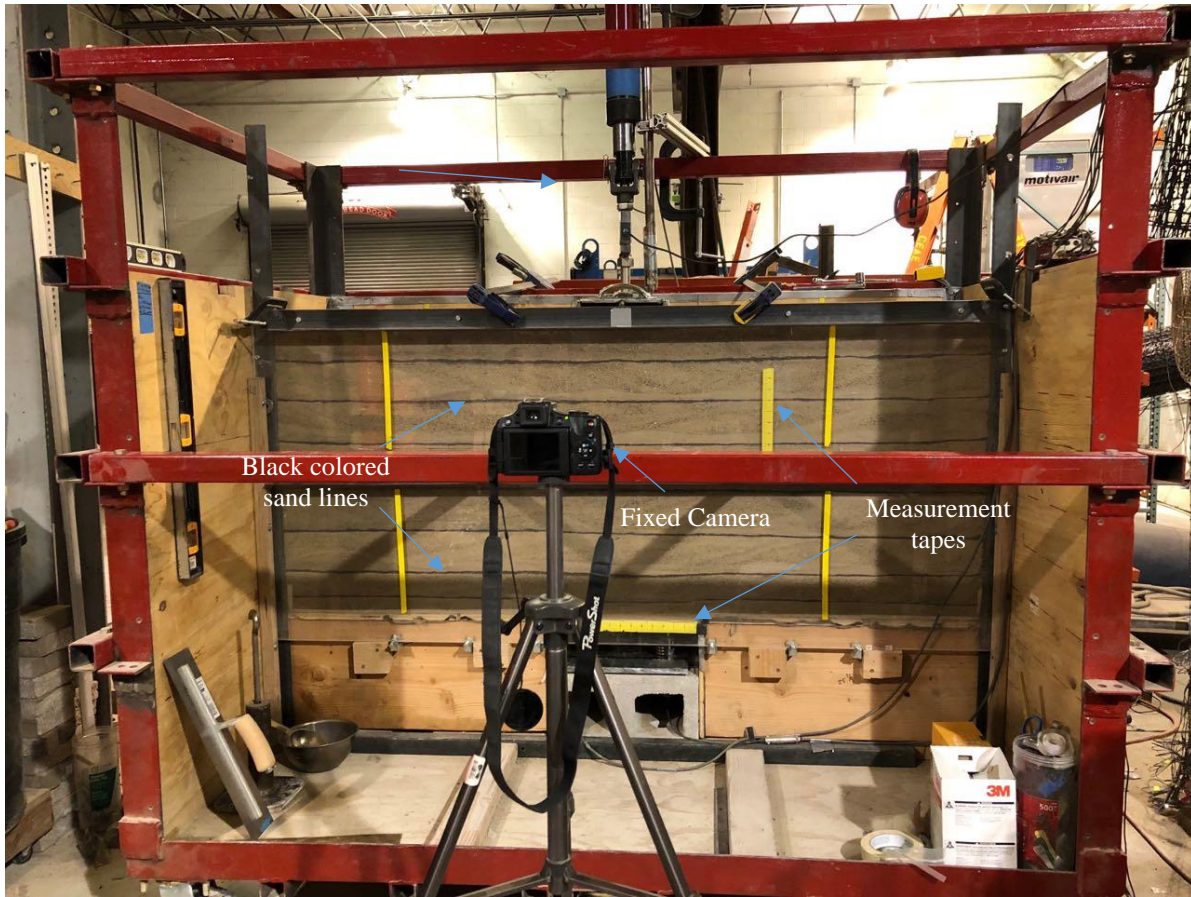
Figure 3.14 Setup for the photogrammetric method.
