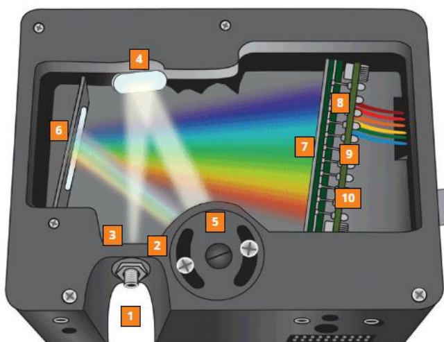
Figure 1.5. Schematics of a commercial miniature spectrometer (USB4000, Ocean Optics, shown in Figure 1.4 ). 1. Optical fiber connector; 2. Entrance slit; 3. Filter; 4. Collimating mirror; 5. Grating; 6. Focusing mirror; 7. Collection lens; 8. Detector; 9. Filter; and 10. Detector window. Reprinted with permission from Ocean Optics.
