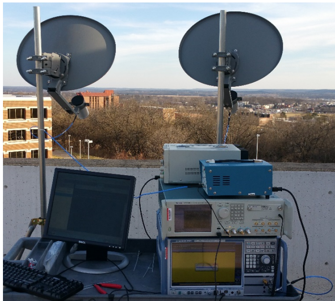
Figure 3.15: Hardware instrumentation setup for open-air measurements
