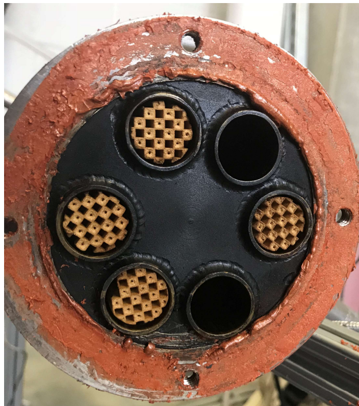
Figure 3.13: DPF cores installed in the HEX after DPFHX testing, showing the slippage of the blocked cores.
