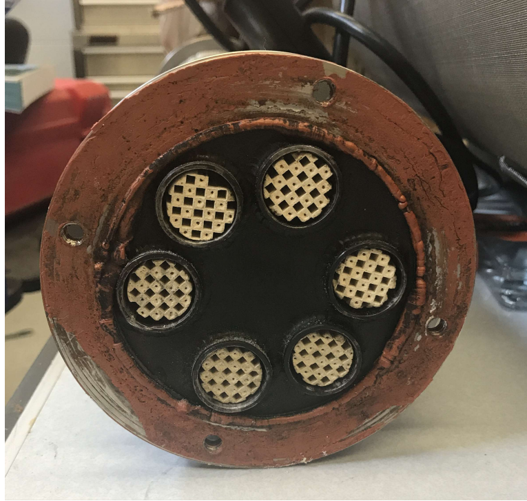
Figure 3.11: DPF cores installed in the six tubes of the HEX.
