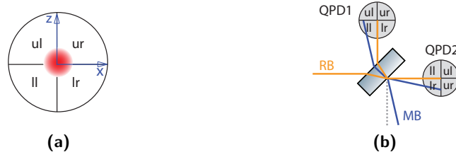
Figure 3.4.: (a) QPD labeling and coordinate system in the direction of beam propagation and (b) illustration of the need of different formulae for the calculation of the DWS and DPS yaw signals.
