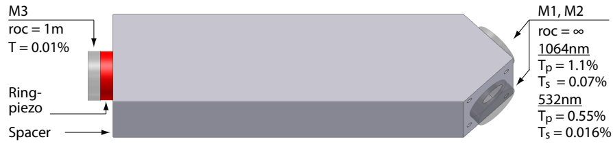
Figure 5.2 — CAD drawing of the mode cleaner cavities MC1064 and MC532. The geometric layout of the spacer and the radius of curvature of M3 was equal for cavities operating at 1064 nm and 532 nm. The cavity round-trip length is 42 cm and the resulting \text{FSR} \approx 714 MHz. The reflectivities of the plane/plane mirrors for different polarization and wavelengths lead to the following values for the Finesse \mathcal{F} and the (FWHM) linewidth \nu . MC1064: \mathcal{F}_p \approx 280 , \nu_p \approx 2.5 MHz, and \mathcal{F}_s \approx 4200 , \nu_s \approx 170 kHz. MC532: \mathcal{F}_p \approx 560 , \nu_p \approx 1.7 MHz, and \mathcal{F}_s \approx 13400 , \nu_s \approx 50 kHz. The spacer for MC1064 was made of aluminum. The spacer for MC532 was made of invar.
