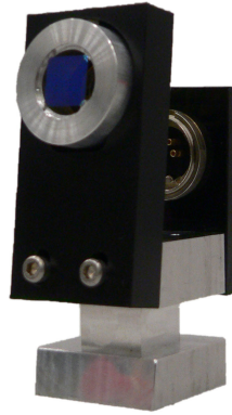
Figure 3.44.: Photograph of a newly designed photo detector mount with polarization filter in front of the photo diode
