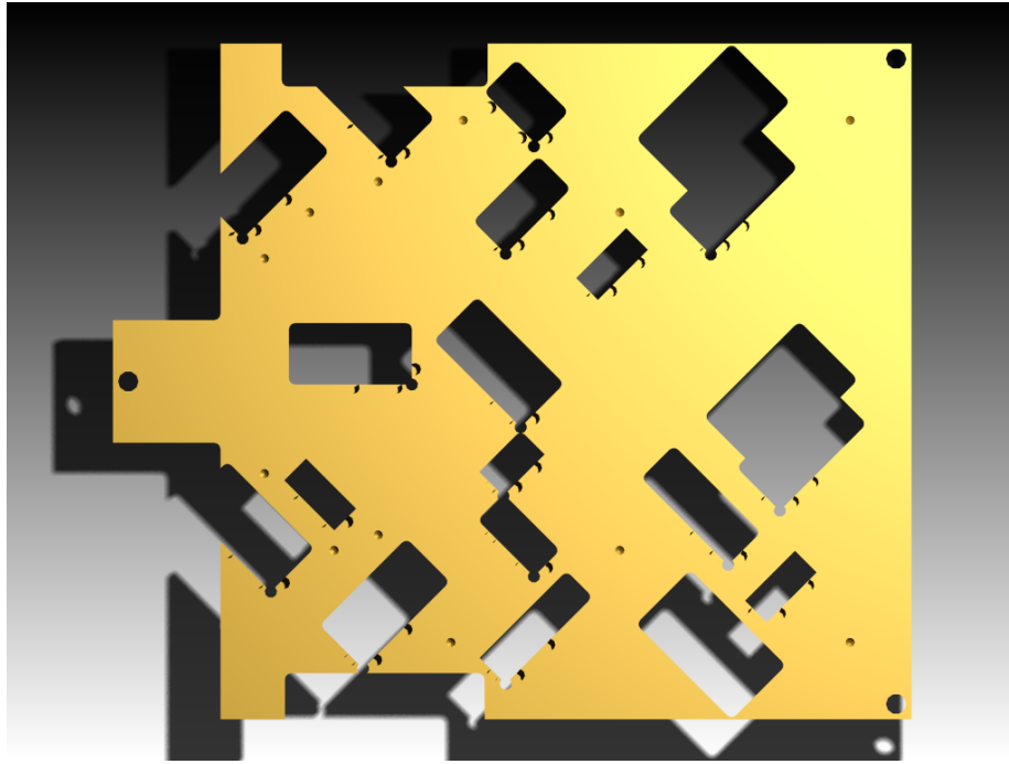
Figure 3.20.: CAD model of the template used to align the optical components on the Zerodur™ base plate
