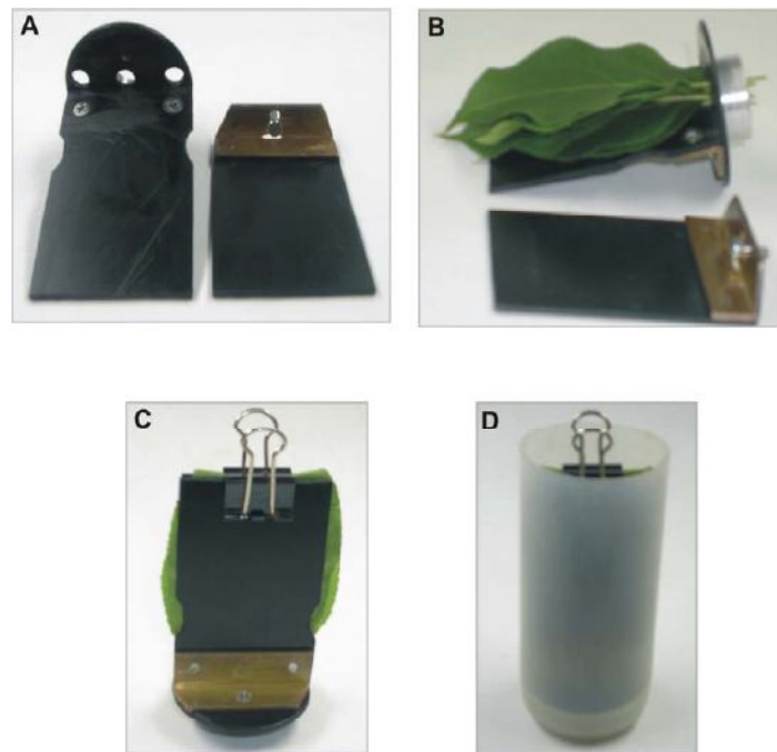
Figure (6): Homemade holder for apoplastic fluid isolation from leaves; A: Holder without plant leaves; B: holder with plant leaves before fixing; C: Fixed plant leaves within the holder; D: Holder with plant leaves, ready for centrifugation (Koutb 2006).
