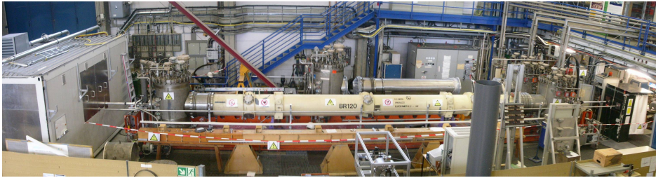
Fig. 3.10: Photo of the complete ALPS I experiment with laser hut (left, light gray), magnet (center, light yellow) and detector cabinet (right, dark green) as it was located in building 55 on the DESY grounds.
