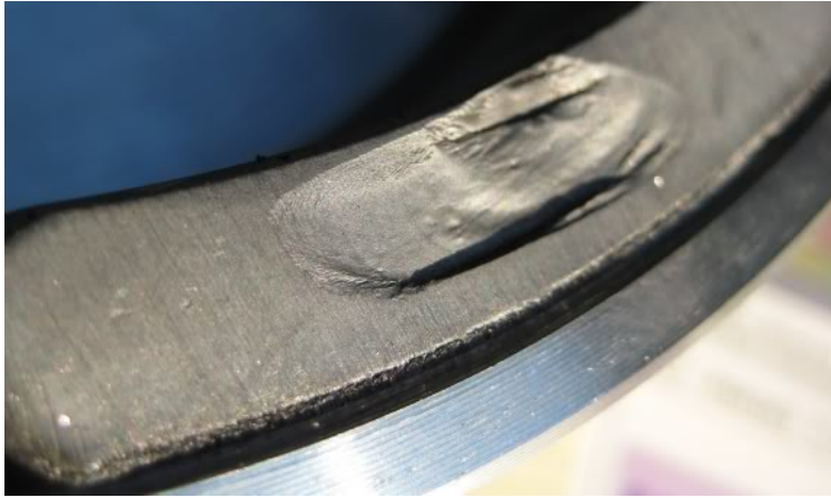
Figure 1.6 A chipped magnet.
