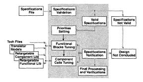
Fig. 4: Retargetable block design flow.
