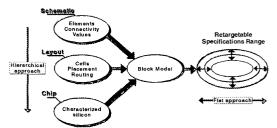
Fig. 3: The concept of block model embeds information from electric schematics, physical layouts and even experimental characterization of a design.
