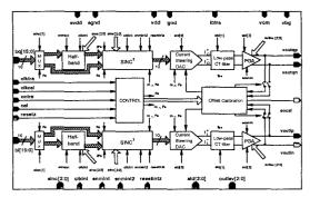
Fig. 2: Block diagram of a mixed-signal block providing full interfacing functionality between a quadrature digital port and a quadrature analog port.
