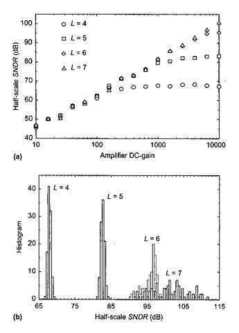
Fig. 3. Effect of (a) finite DC-gain and (b) weight mismatch on SNDR for M = 16.
