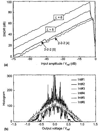
Fig. 2. (a) *SNDR* vs. input level under ideal conditions. (b) Histograms of the integrator outputs relative to the reference voltage.
