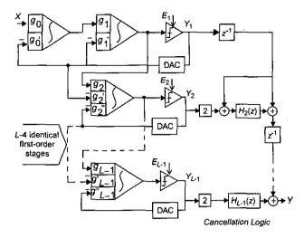
Fig. 1. Lth-order 2-1<sup>L-2</sup>  $\Sigma \Delta M$ .  $H_k(z) = (1 - z^{-1})^k$ , k = 2...L - 1
